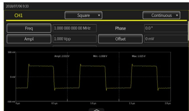
Figure 17. AFG31000 Series InstaView display user interface
