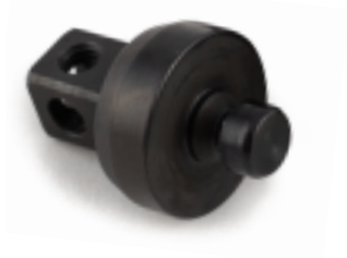
104512 - QC Adapter 4side block, bores M5, M6 + M5 inner thread
