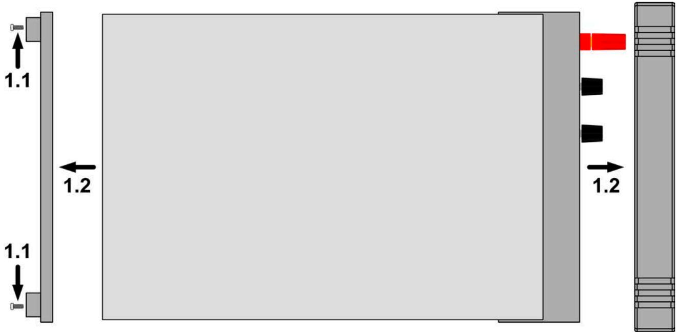
Figure 7 - Removal of the front and rear frame
