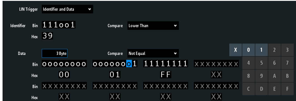
Figure 13-32: Trigger setup to trigger on identifier and data patterns
