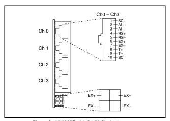
Figure 2. NI 9237E with RJ-50 Pin Assignments
