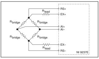
Figure 5. Connecting Remote Sense Wires to the NI 9237E
