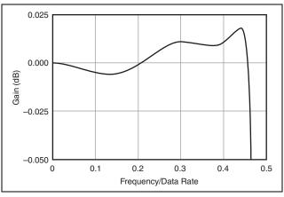
Figure 6. Typical Passband Flatness for the NI 9237E
