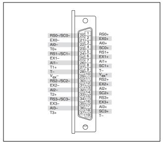
Figure 3. NI 9237E with DSUB Pin Assignments
