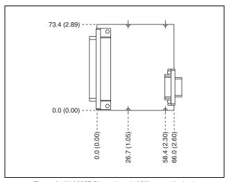
Figure 1. NI 9237E Dimensions in Millimeters (Inches)
