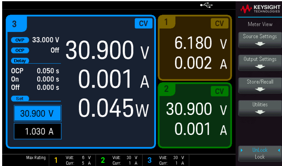
Figure 2. View details of a single channel including the measured power, OVP/OCP condition, and delays.
