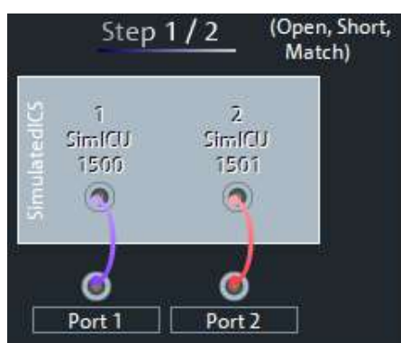
Figure 10-16: Automatic calibration: inline calibration system
