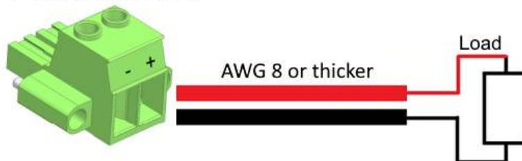
*Figure 3-7: Connection to load*
