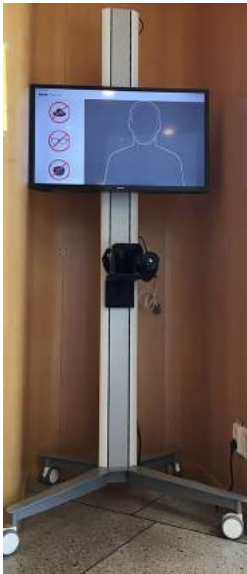
Figure 3.2 Stand with rail for flexible mounting of display and camera
