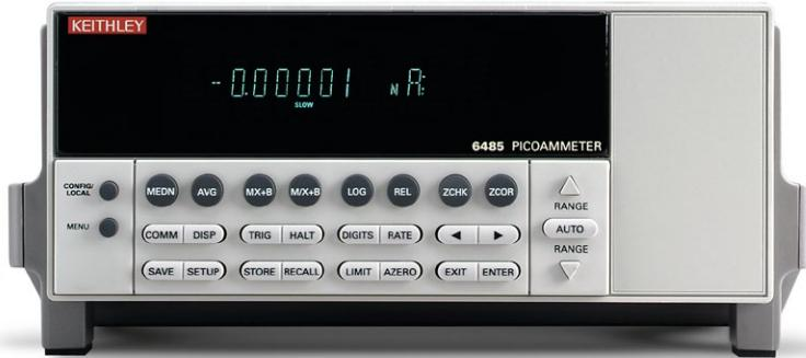
The 5½-digit 6485 Picoammeter combines Keithley's expertise in sensitive current measurement instrumentation with enhanced speed and a robust design. With eight current measurement ranges and high speed autoranging, this cost-effective instrument can measure currents from 20 fA to 20 mA, taking measurements at speeds up to 1000 readings per second.
