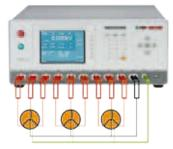
Y-type motor for example, the test items are: •HSCC / OSC •DCR Test Impulse Test •Hi-pot –Sub step test
