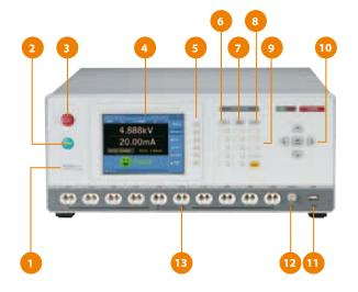
1.Power switch 2.Start button 3.Stop button 4.LCD color display 5.Function key 6.Test key 7.Main index key
