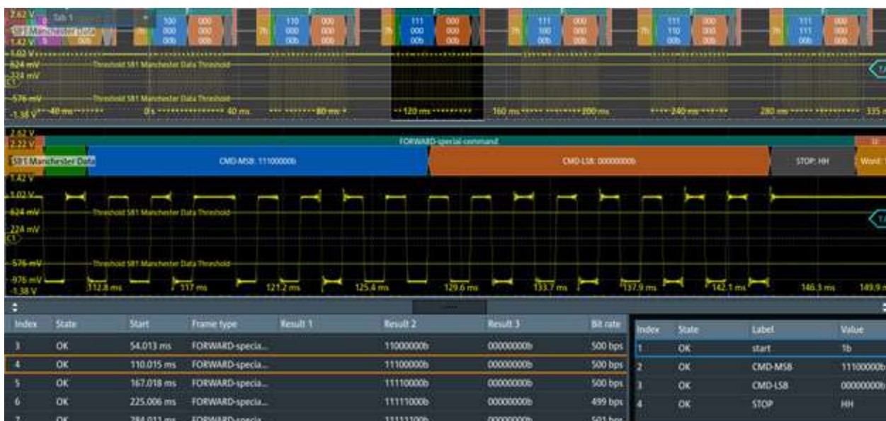
Figure 14-27: Decoded Manchester signal
