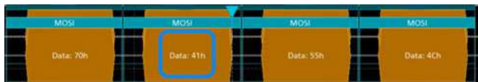
Figure 14-9: Trigger on Type= MOSI, Data pattern = 41
