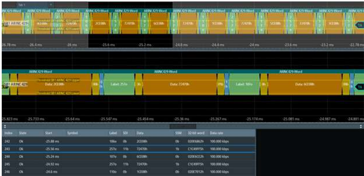
Figure 14-38: Decoded ARINC429 signal
