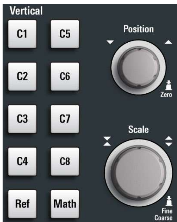
Figure 3-5: Vertical controls of MXO 5 with 8 input channels
