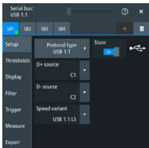
Figure 14-59: Serial bus protocol configuration dialog for USB 1.1 LS or FS
