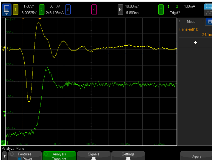
Figure 8. Transient response settling time measurement.
