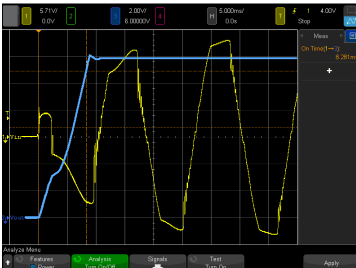
Figure 7. AC-to-DC turn-on time measurement.
