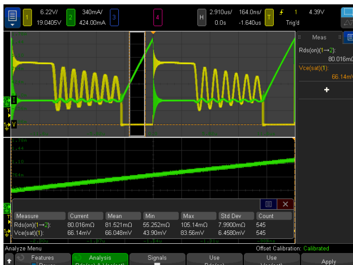
Figure 4. R_{DS(ON)} and V_{CE(SAT)} measurements.
