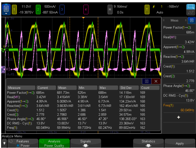
Figure 1. Input AC power quality measurements.
