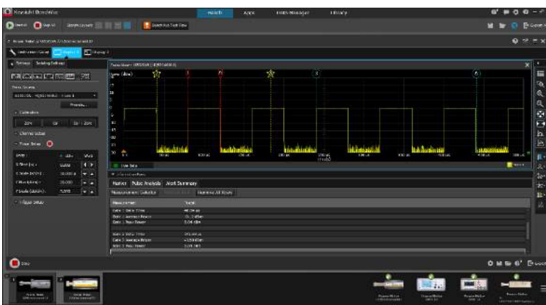
Multi-channel trace display with 4-pairs of gates and automatic pulse parameters measurement
