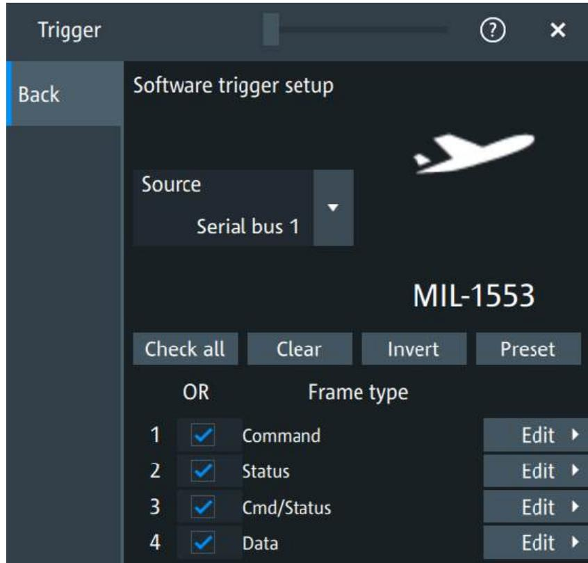
In the "Software Trigger" tab, you can define the settings to trigger on the frames that match the selected filter conditions.
