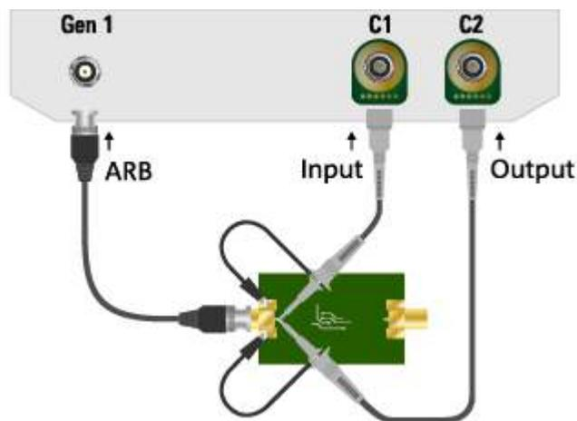
**Figure 12-4: Example of a calibration test setup**
