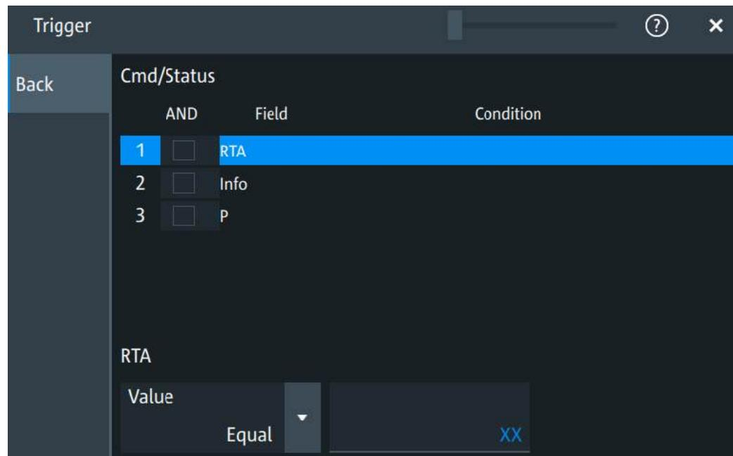
"Field" Enables the field type that you want to trigger on for the selected frame.
