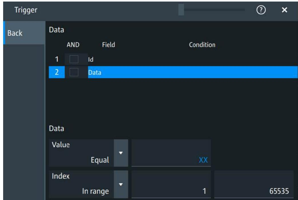
"Field" Enables the field type that you want to trigger on for the selected frame.
