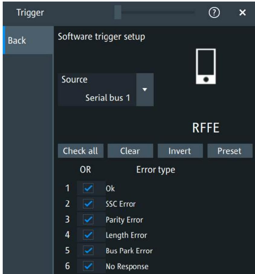
The following error types are available: "OK", "SSC Error", "Parity error", "Length error", "Bus park error", "No response".
