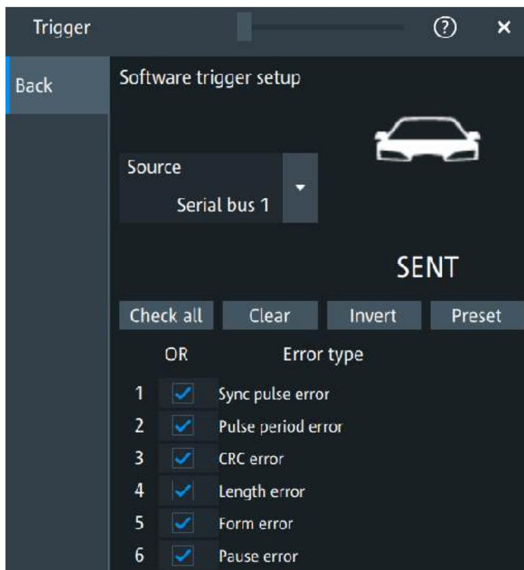
The following error types are available: "Sync pulse error", "Pulse period error", "CRC error", "Length error", "Form error", "Pause error".
