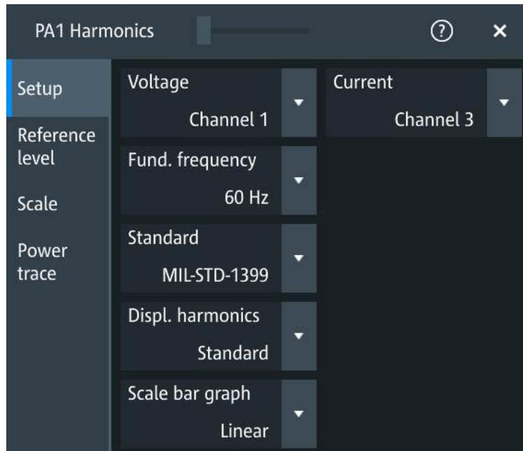
Figure 12-8: Power harmonic setup for MIL-STD-1399/ RTCA DO-160
