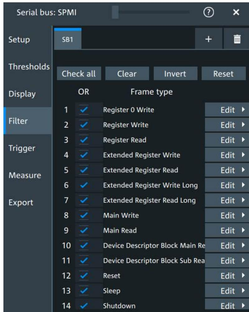
In the "Filter" tab, you can define the settings to display only the frames that match the selected filter conditions.
