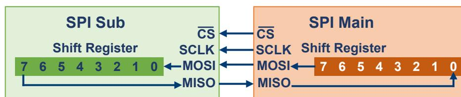
Figure 14-7: Simple configuration of SPI bus
