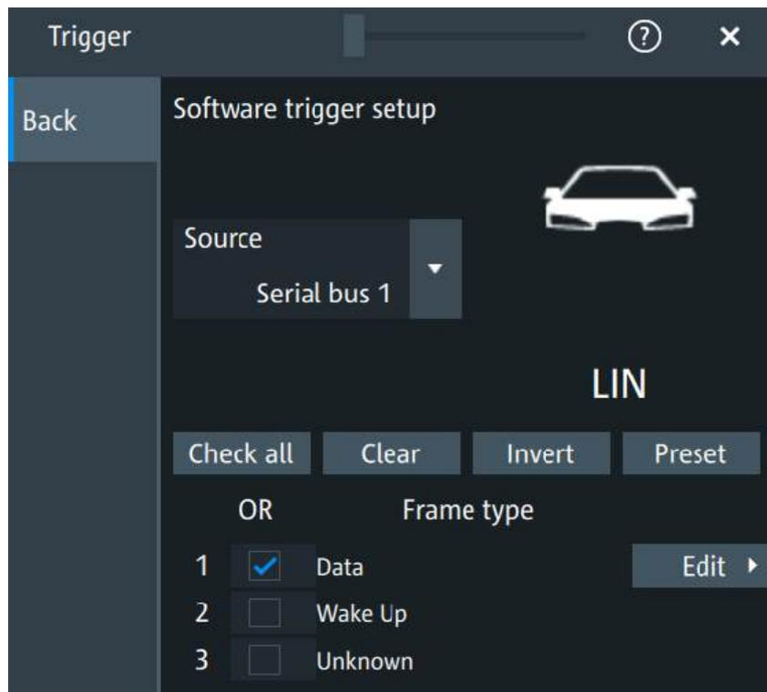
In the "Software Trigger" tab, you can define the settings to trigger on the frames that match the selected filter conditions.
