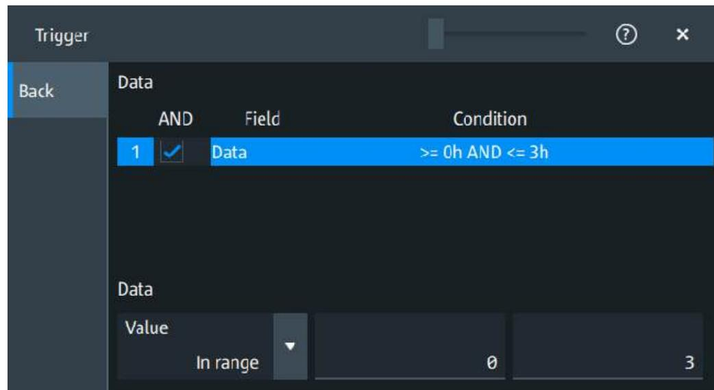
"Field" Enables the field type that you want to trigger on for the selected frame.
