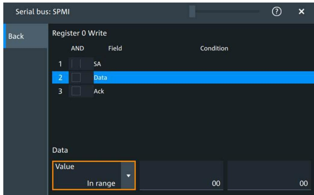
"Field" Enables the field type that you want to filter on for the selected frame. The available fields depend on the selected frame type.
