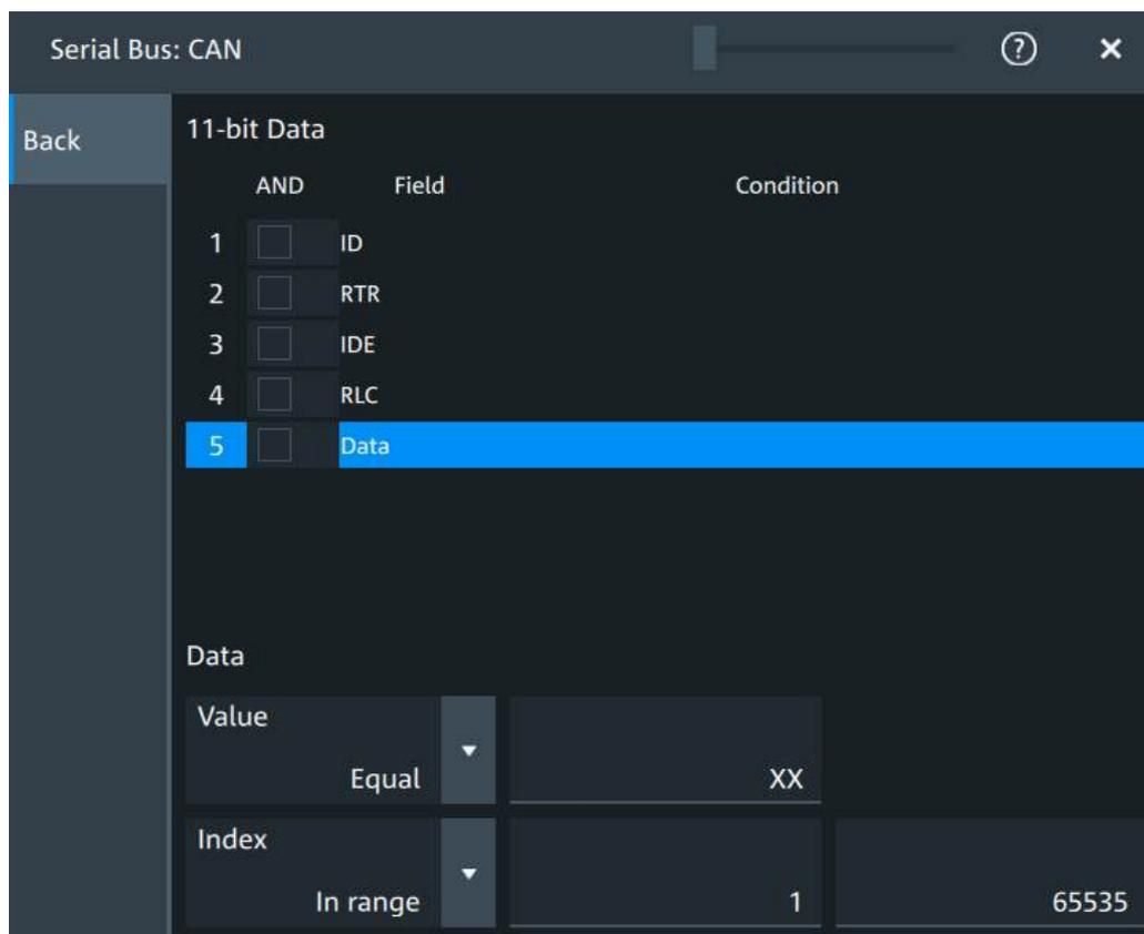
"Field" Enables the field type that you want to filter on for the selected frame. The available fields are "ID", "RTR", "ITE", "RLC" and "Data".
