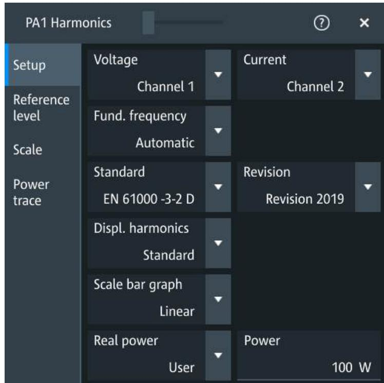
Figure 12-7: Power harmonic setup for EN 61000-3-2 D
