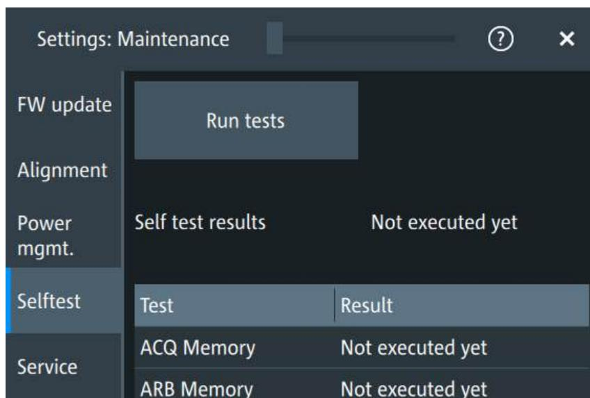
The selftest can take several minutes. The summary result is shown in the "Selftest results" field, and the results of the single tests are shown in the "Result" column of the test table.
