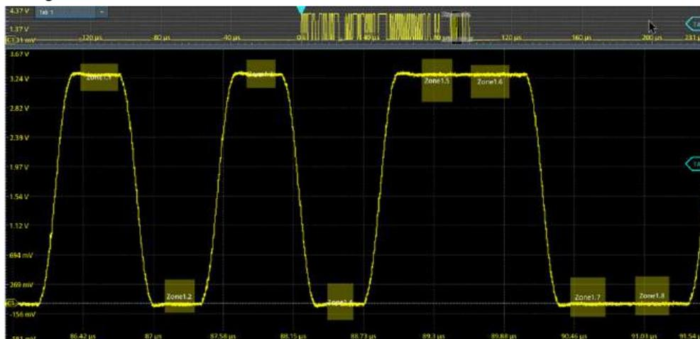
Figure 7-7: Zone trigger on digital serial pattern
