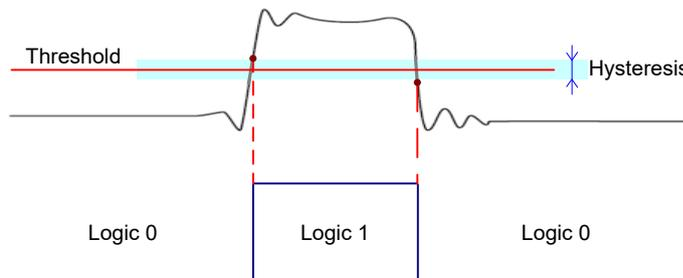
By default, the same threshold and hysteresis value are used for all digital channels and all logic buses: "Couple thresholds" is enabled.
