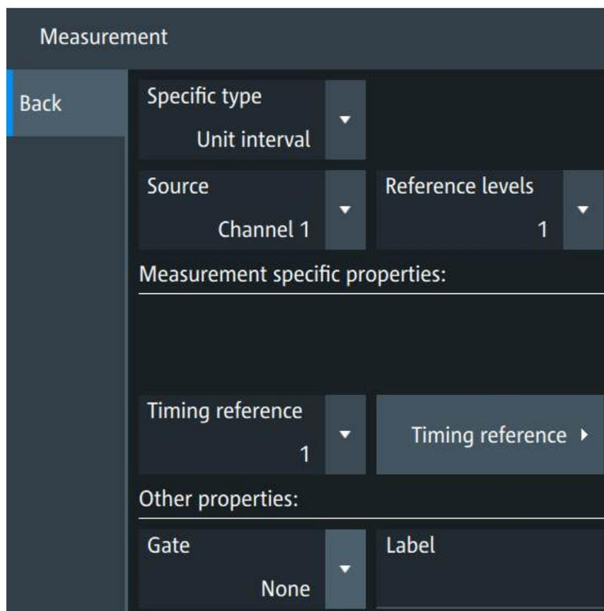
Figure 10-2: Setup for unit interval measurement
