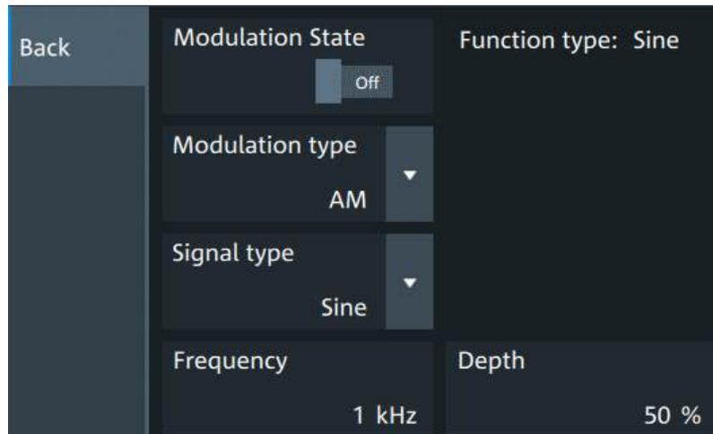
Figure 16-1: Modulation setup
