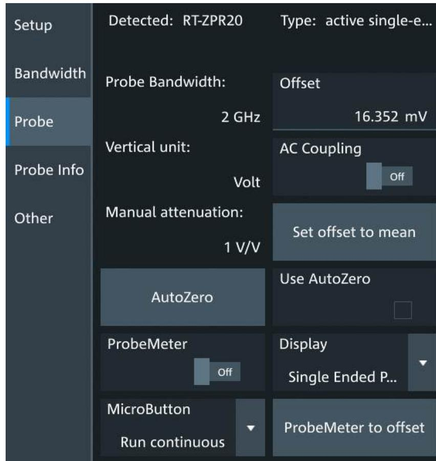
Figure 6-5: Probe setup for power rail probe R&S RT-ZPR20
