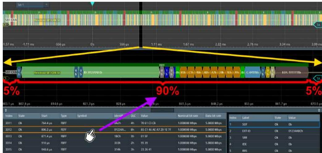
**Figure 14-3: Zoom coupling of selected frame (left table)**
