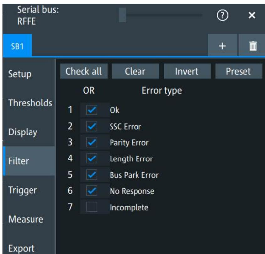
The following error types are available: "OK", "SSC Error", "Parity error", "Length error", "Bus park error", "No response".
