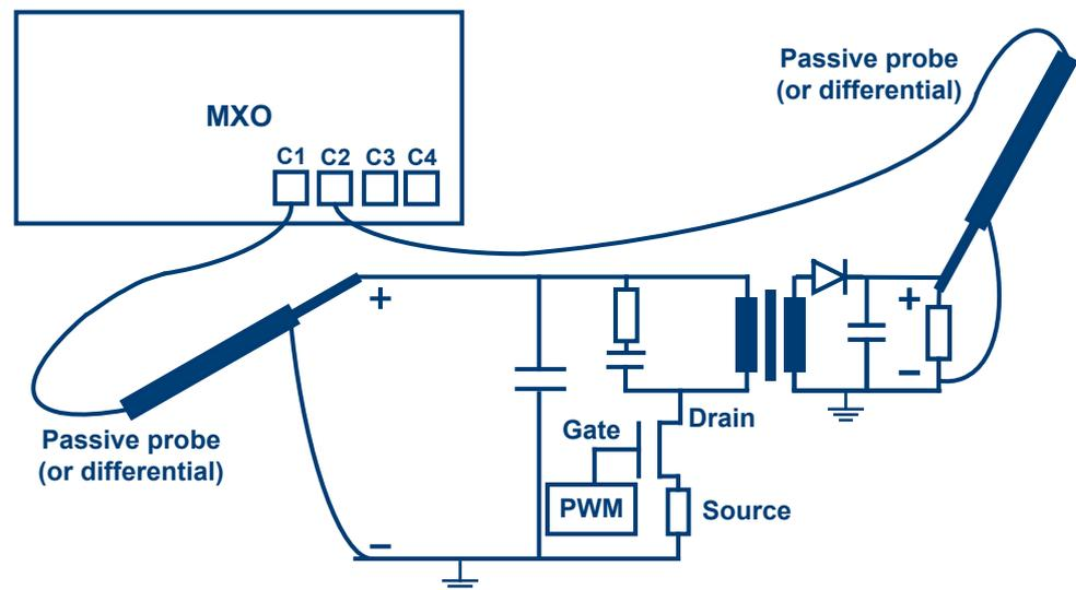
Figure 12-10: Connection with DC input
