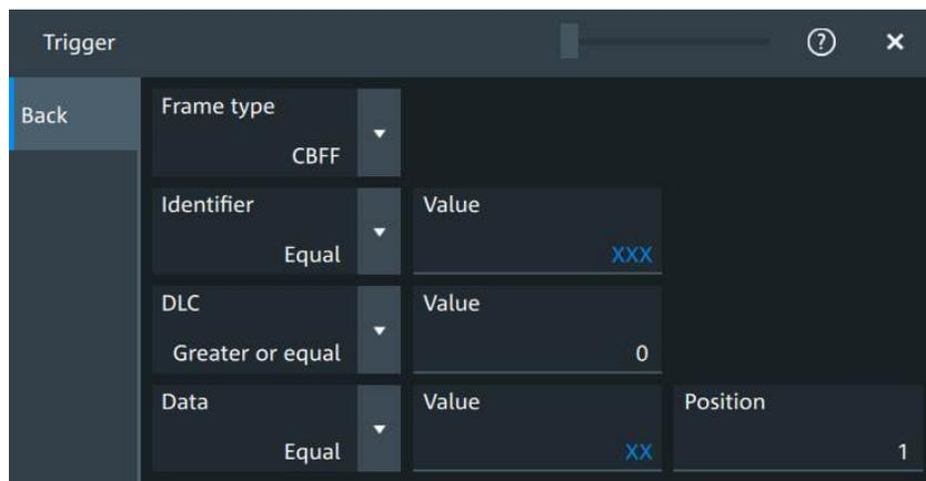
"Identifier" Sets the trigger to a specific message identifier or an identifier range.
