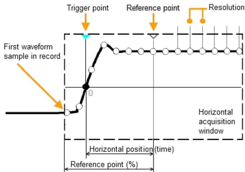
Unlike vertical settings, which are waveform-specific, the horizontal settings apply to all active waveforms.
