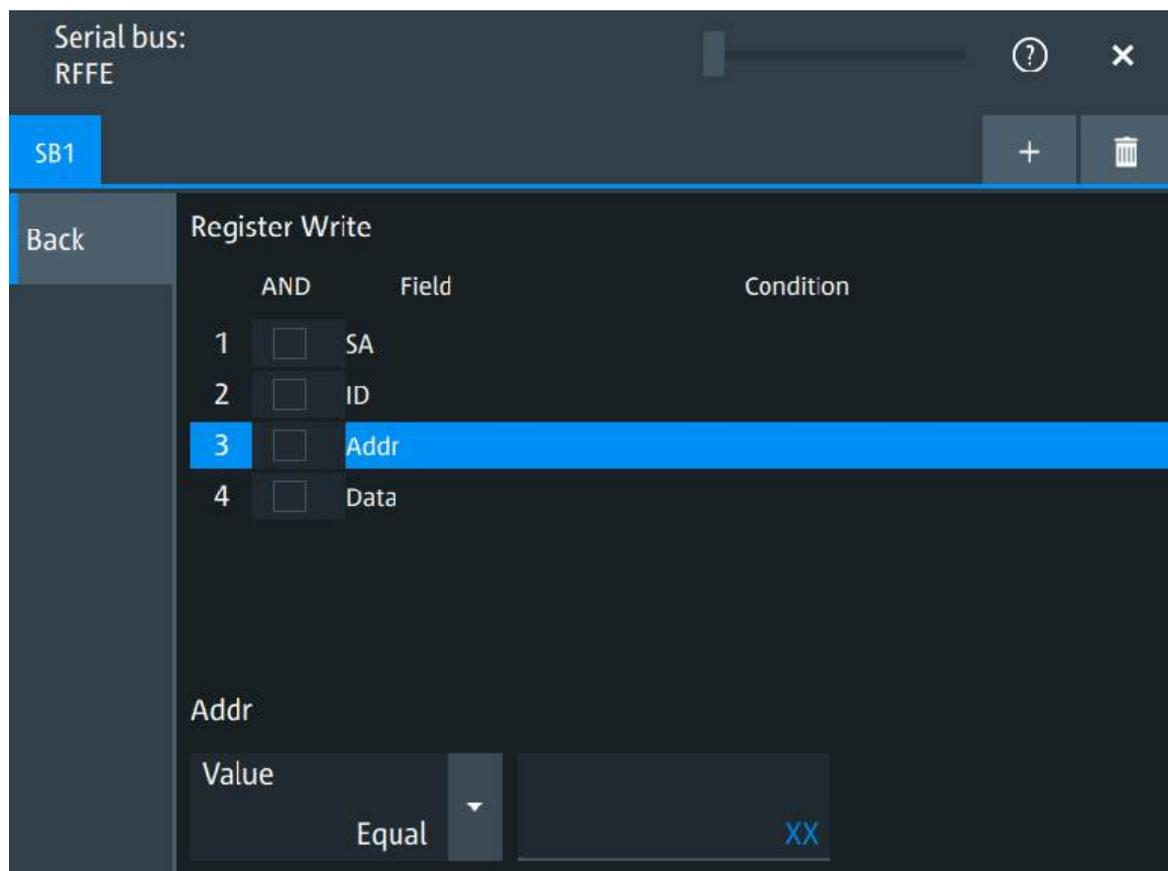
"Field" Enables the field type that you want to filter on for the selected frame. The following fields are available: "SA", "ID", "Data", "Addr", "BC", "MID", "Data MSB", "Data LSB".
