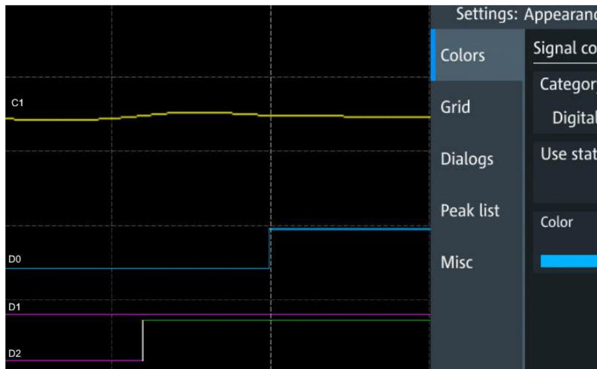
*Figure 5-1: D0 has a selected color (blue). D1 and D2 have state coloring. D1 is on low level, D2 changes from low to high.*
