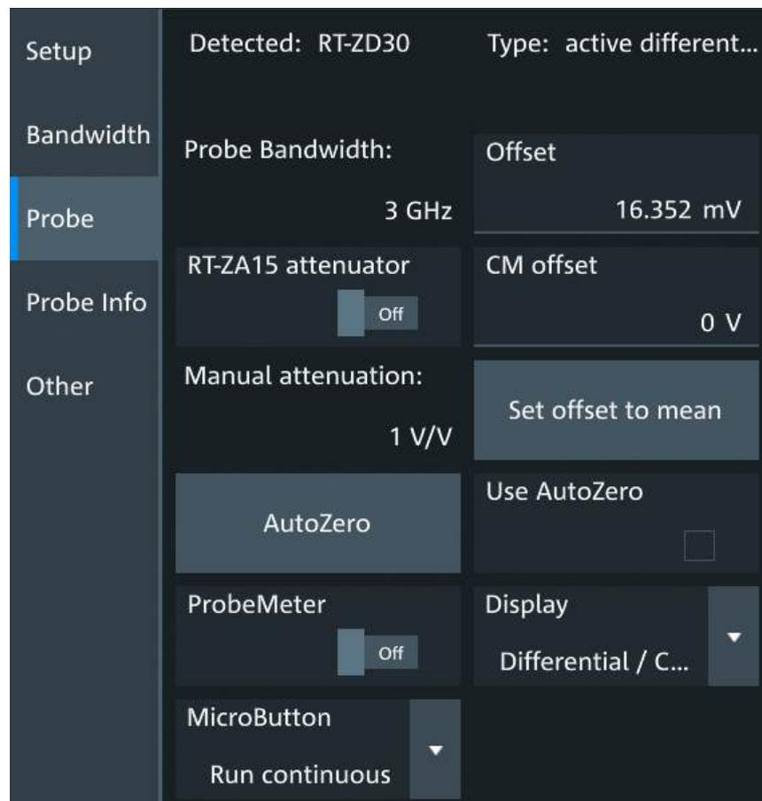
Figure 6-4: Probe setup for active differential probe R&S RT-ZD30
