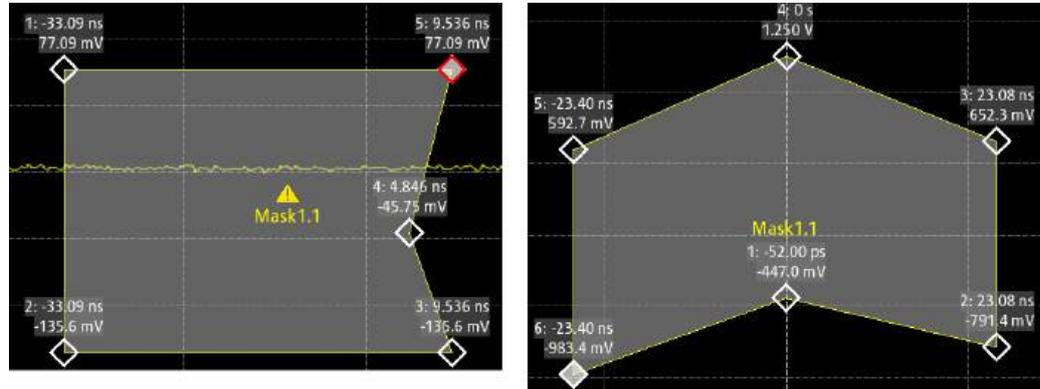
Figure 12-1: Invalid mask segment (left) and valid mask segment (right)
