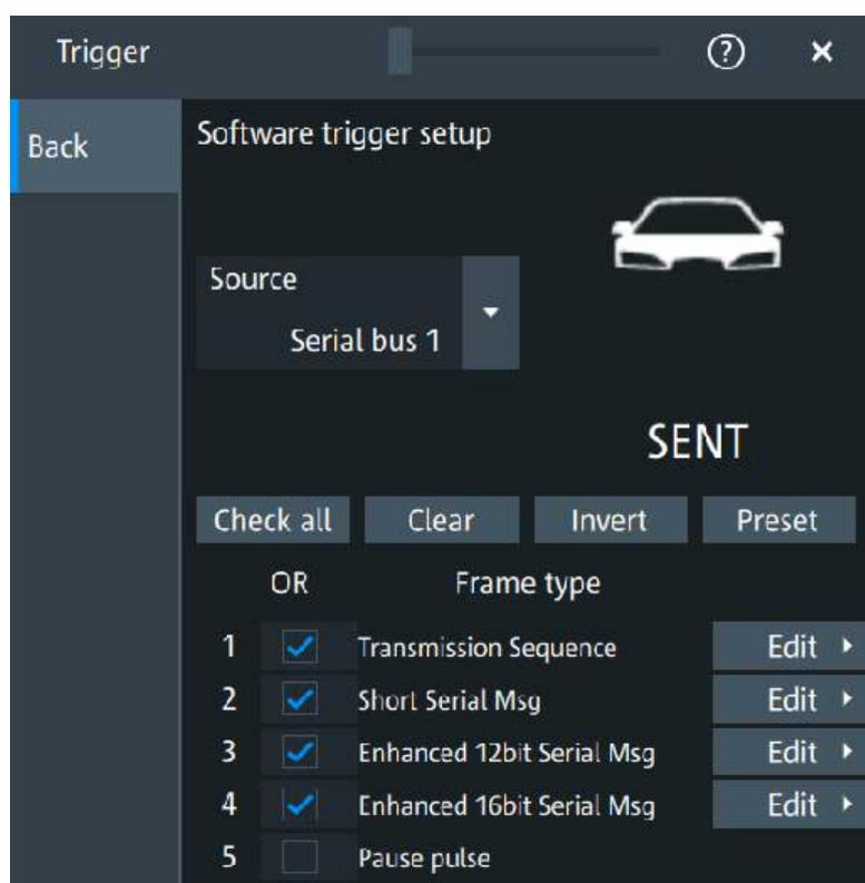
In the "Software Trigger" tab, you can define the settings to trigger on the frames that match the selected filter conditions.
