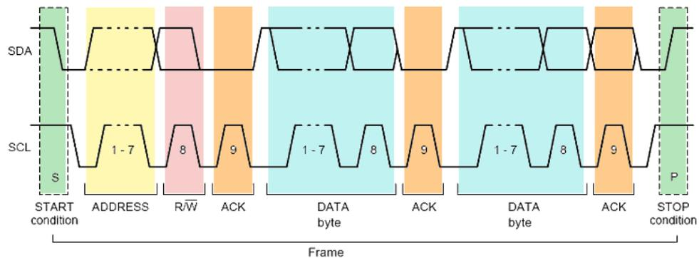
Figure 14-11: I<sup>2</sup>C write access with a 7-bit address
