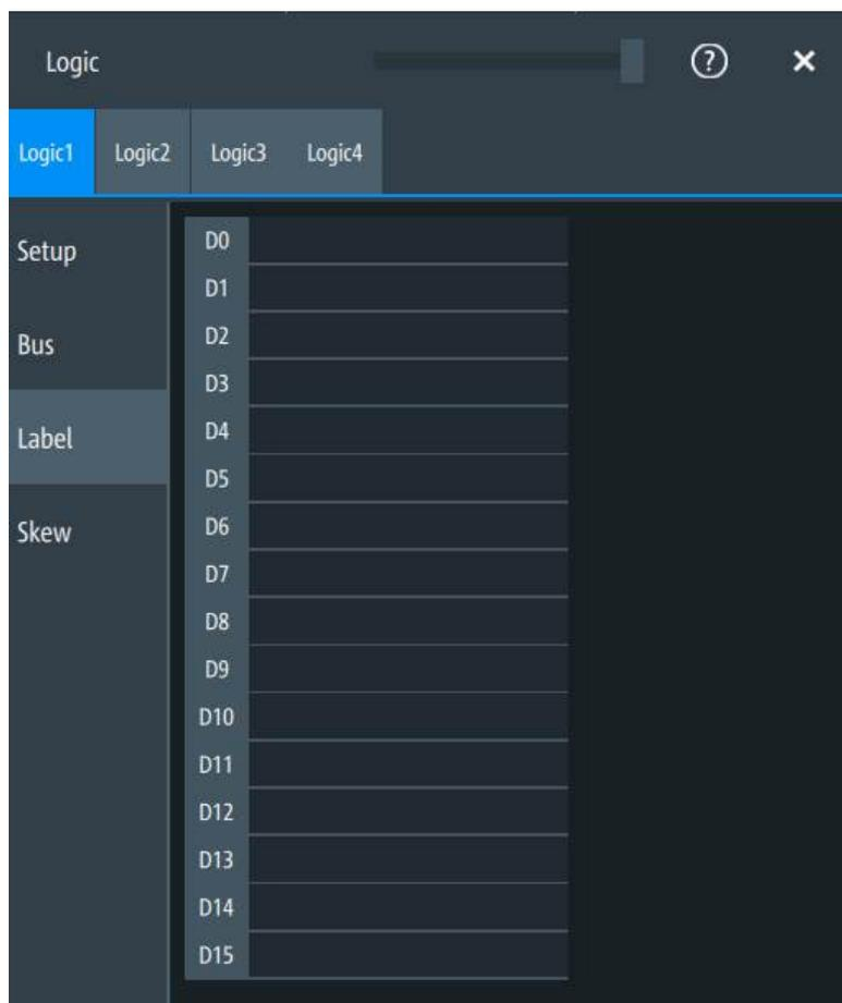
In this tab, you can enter a name for each digital channel. The name is displayed in the diagram.
