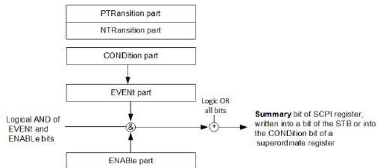
The five parts of a SCPI status register have different properties and functions:
