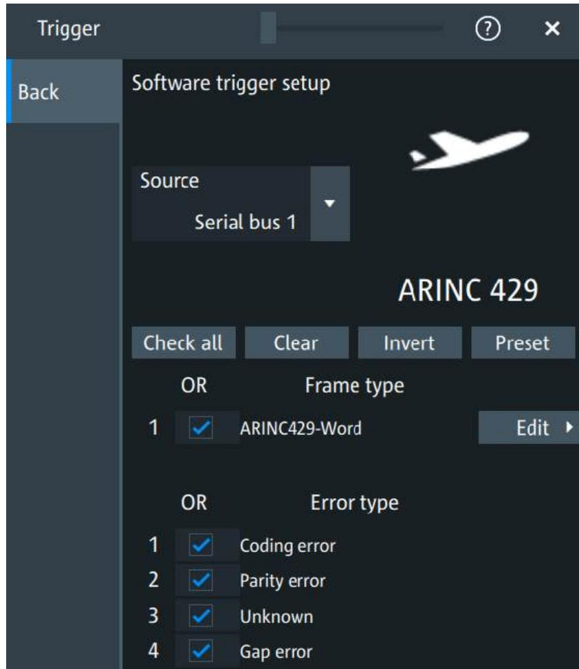
In the "Software Trigger" tab, you can define the settings to trigger on the frames that match the selected filter conditions.
