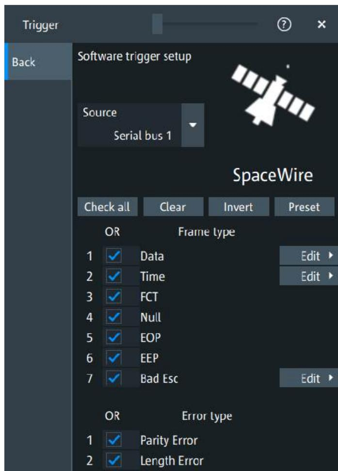
In the "Software Trigger" tab, you can define the settings to trigger on the frames that match the selected filter conditions.
