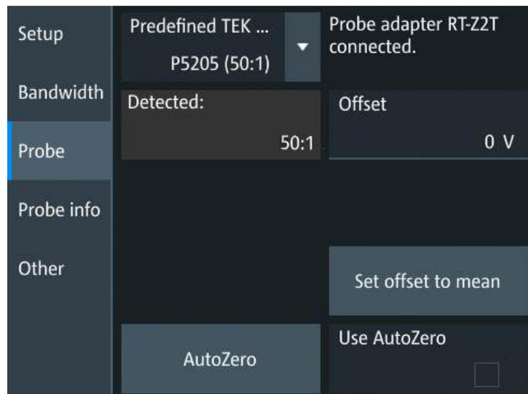
The dialog shows that the R&S RT-Z2T probe interface adapter is connected, and supported Tektronix probes are listed as "Predefined probe".
