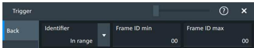
"Identifier + Data" Sets the trigger to a combination of identifier and data condition. The instrument triggers at the end of the last byte of the specified data pattern.
