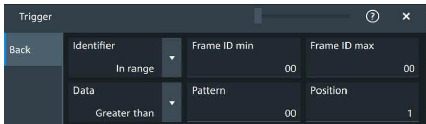
The identifier conditions are the same as for the "Identifier" trigger type, see [Identifier setup: Condition, Frame ID min, Frame ID max.](#) Data conditions are set with [Data setup: Condition, Pattern, Position.](#)
