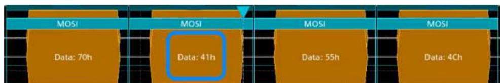
Figure 14-9: Trigger on Type= MOSI, Data pattern = 41
