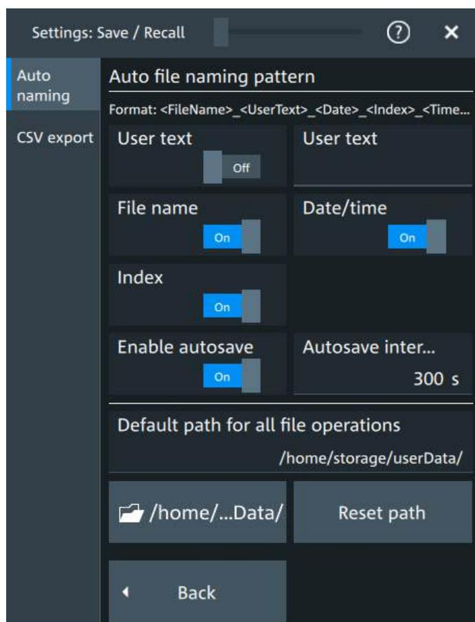
In the "Autonaming" tab, you can define the pattern for automatic filename generation. This name is used as the default filename. The default path is the storage location for all saved files and their subdirectories. The local directory for user data is `/home/storage/userData`, the path to a USB storage device is `/run/media/usb/<MyDriveName>/`.
