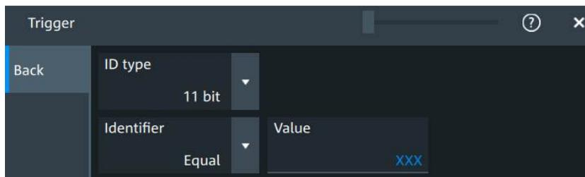
"Identifier + Data" Sets the trigger to a combination of identifier and data condition. The instrument triggers at the end of the last byte of the specified data pattern.
