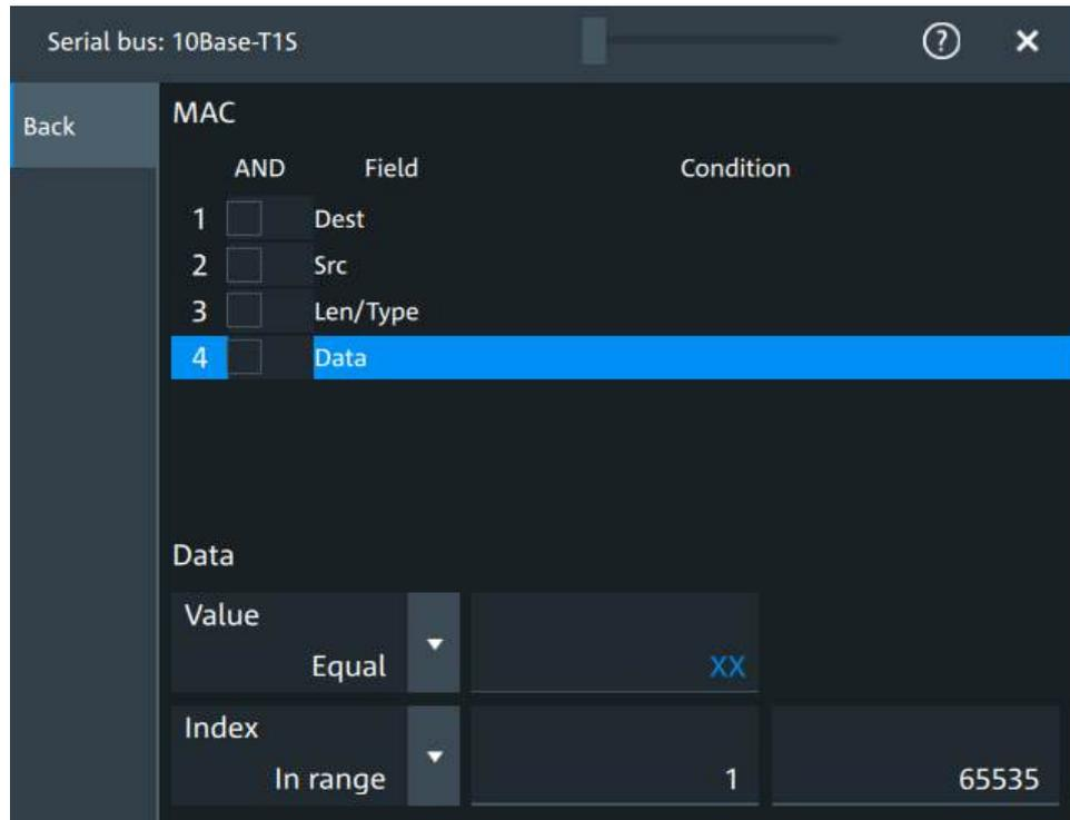
"Field" Enables the field type that you want to filter on for the selected frame. The available fields are "Dest", "Src", "Len/Type" and "Data".
