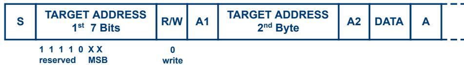
Figure 14-12: 10-bit address, write access
