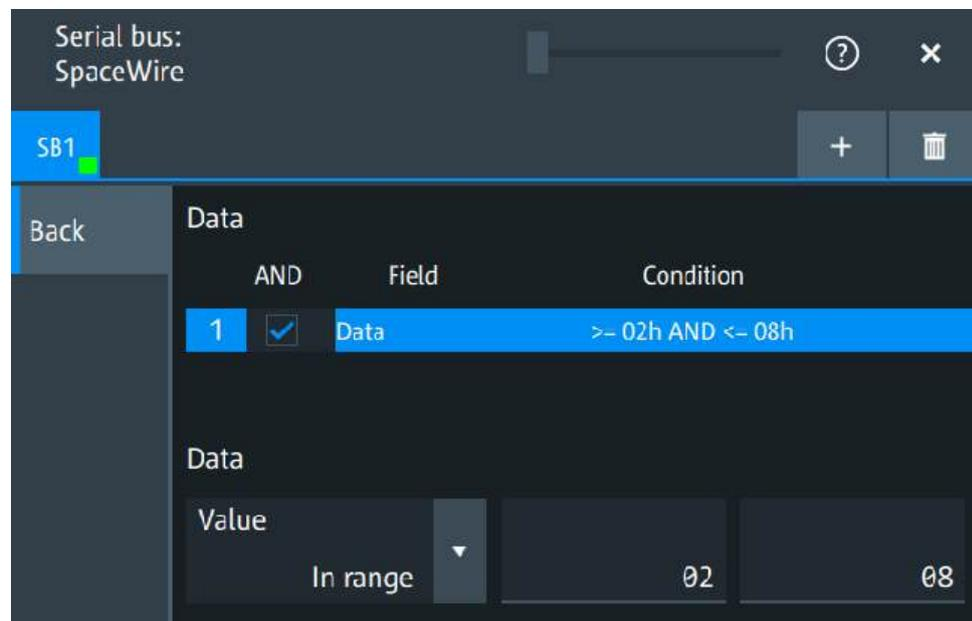
"Field" Enables the field type that you want to filter on for the selected frame. The available fields are "Data", "Time", "Bad Esc".
