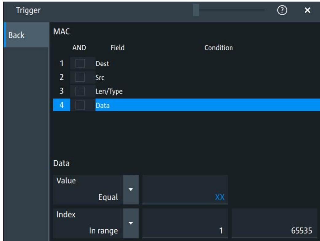
"Field" Enables the field type that you want to trigger on for the selected frame.
