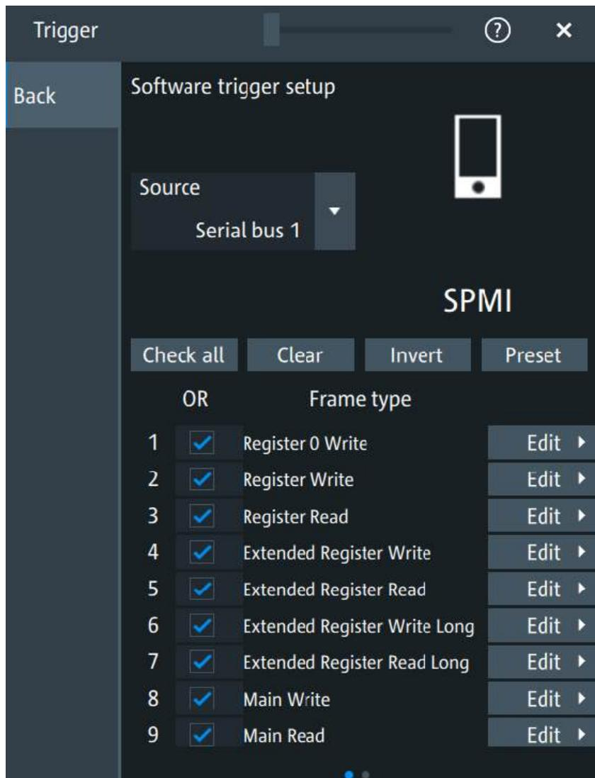
In the "Software Trigger" tab, you can define the settings to trigger on the frames that match the selected filter conditions.
