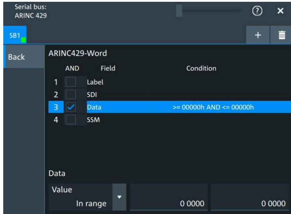
"Field" Enables the field type that you want to filter on for the selected frame. The available fields are "Label", "SDI", "Data", "SSM".
