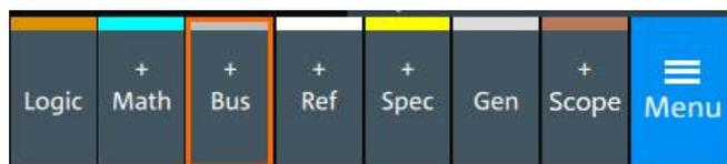
2. Select the tab of the bus that you want to set up, for example "SB1".
