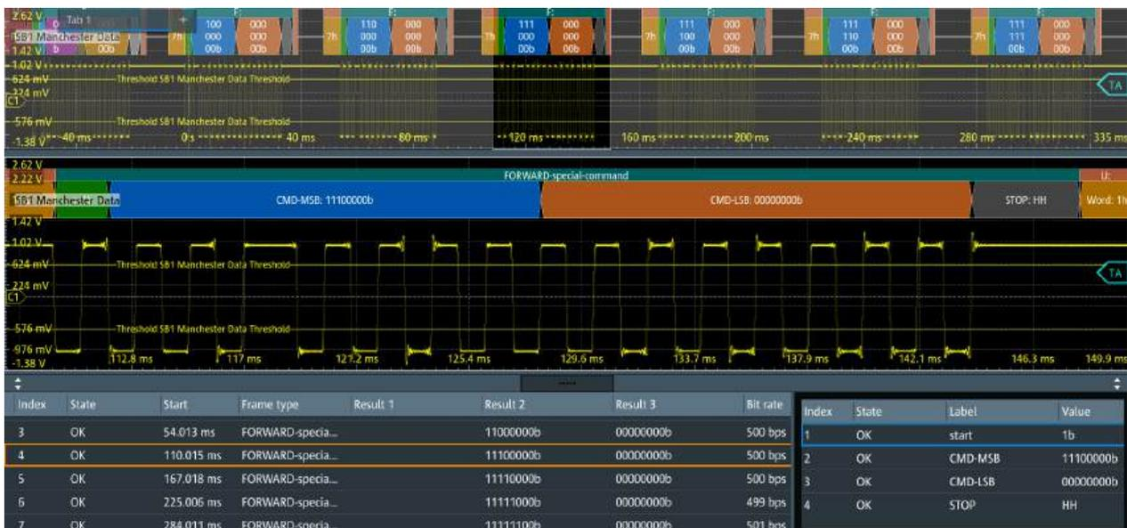
**Figure 14-27: Decoded Manchester signal**
