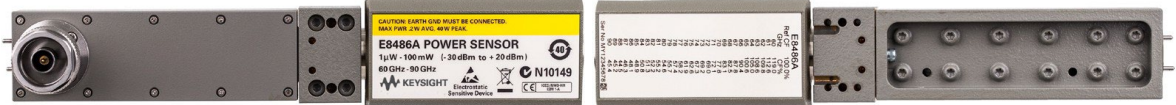
Figure 1. E8486A-100 comes without built-in EEPROM with a dynamic range of -30 to +20 dBm. Users need to pre-enter calibration factors printed on the back of the sensor into the power meter.
