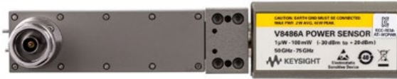
Figure 3. V8486A-100 comes without built-in EEPROM. Users need to pre-enter calibration factors printed on the back of the sensor into the power meter.
