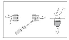
Figure 2-5 Removing the feet from the cover.
