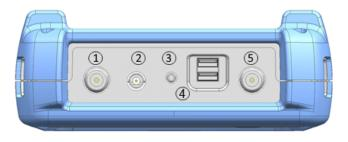
1 = RF input 2 = BNC connector 3 = Headphone jack 4 = USB type A connector 5 = RF output
