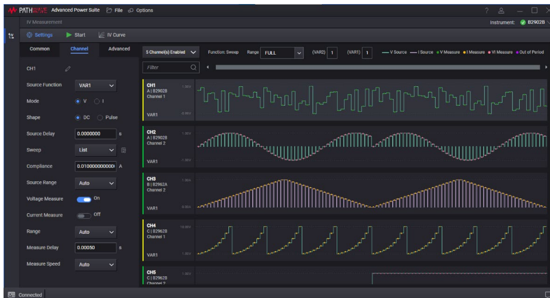
Figure 1. Previewing the settings of multiple SMU channels
