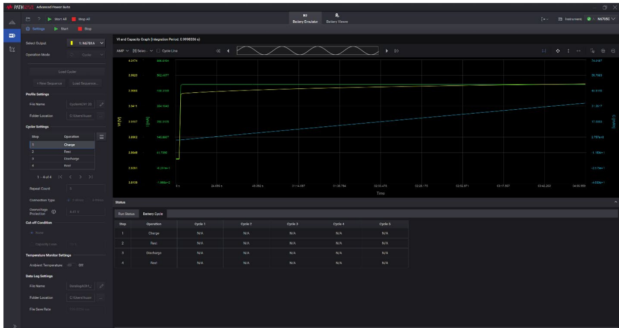
Figure 12. PW9254A Cycle testing a 18650 battery
