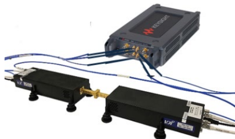
E-band VNA solution using P502xA and N5252AW frequency extenders.
