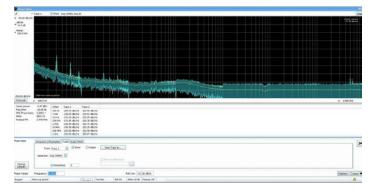
The RSA7100B's intrinsic phase noise of -134 dBc/Hz, at this frequency and across its operating range, provides ample measurement margin for a vast majority of applications.
