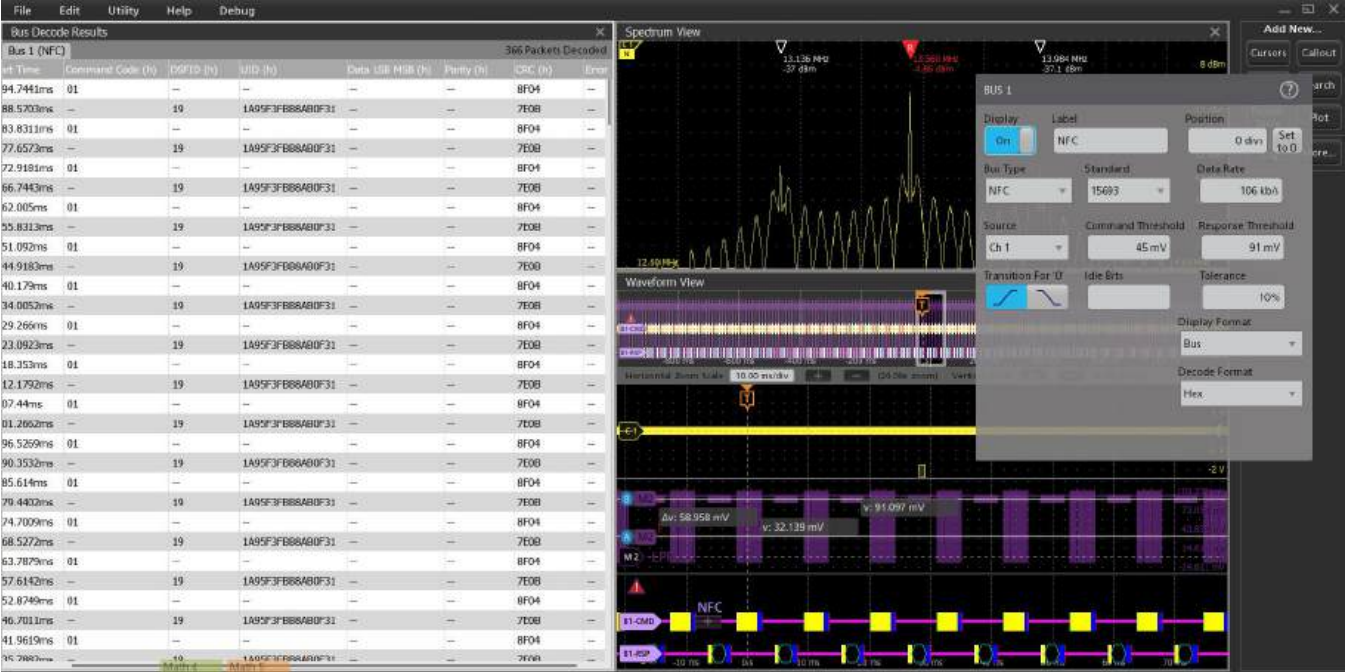
NFC software option allows you to decode and search through their digital NFC bit stream for performing NFC analog/RF and digital pre-conformance, debug, and troubleshooting in a single instrument.
