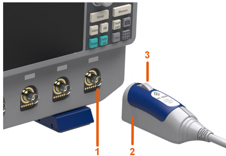
Figure 3-1: Connecting the probe to the Rohde & Schwarz oscilloscope
