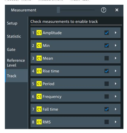
Figure 9-5: Measurement selection for tracks
