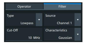
The finite impulse response filter is a filter to create filtered math waveforms with low-pass or highpass. The filter requires additional settings.
