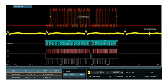
Figure 13-3: Decoded and binary SPI signal
