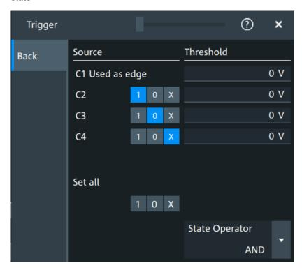
Figure 7-2: Set state for state trigger
