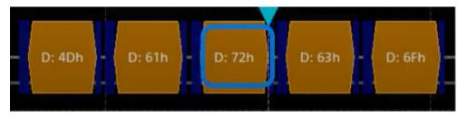
Figure 13-12: Trigger on Type= Tx, Data =0x72 and Position=3
