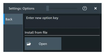
In the "Install" tab, you can install new options using license keys.
