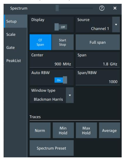
In this tab, you define the settings for the spectrum window. The display can be restricted to the results for a certain time base extract and to a specified frequency range.
