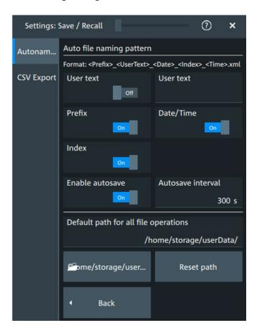
In the "Autonaming" tab, you can define the pattern for automatic file name generation. This name is used as the default file name. The default path is the storage location for all saved files and their subdirectories. The directory for user data on the instrument is /home/storage/userData, the path to a USB storage device is /run/media/usb/.
