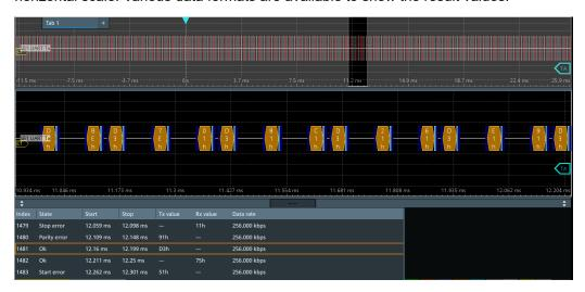
Figure 13-11: Decoded and binary UART signal
