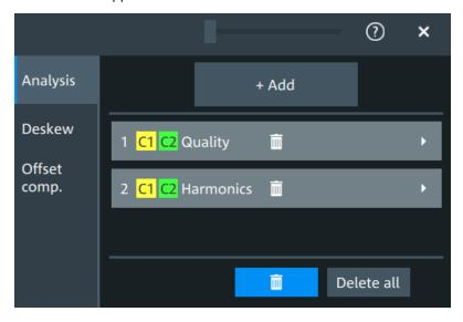
3. Tap on the button of the power measurement that you want to delete. Alternatively, tap "Delete All" to delete all measurements.
