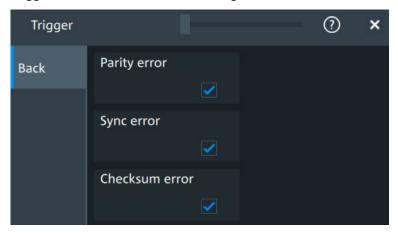
"Parity error" Parity bits are the bits 6 and 7 of the identifier. They verify the correct
