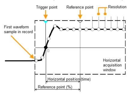
Unlike vertical settings, which are waveform-specific, the horizontal settings apply to all active waveforms.
