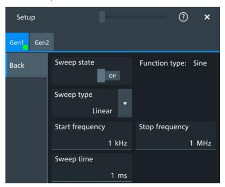
In the sweep mode, the R&S MXO 4 generates a signal whose frequency gradually changes from the "Start frequency" to the "Stop frequency" for a certain "Sweep time".
