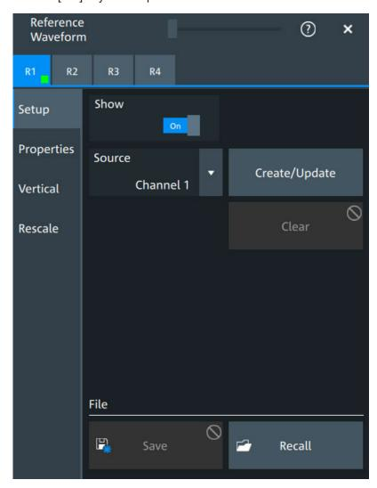
In the "Setup" tab, you select the target reference waveform and its source.
