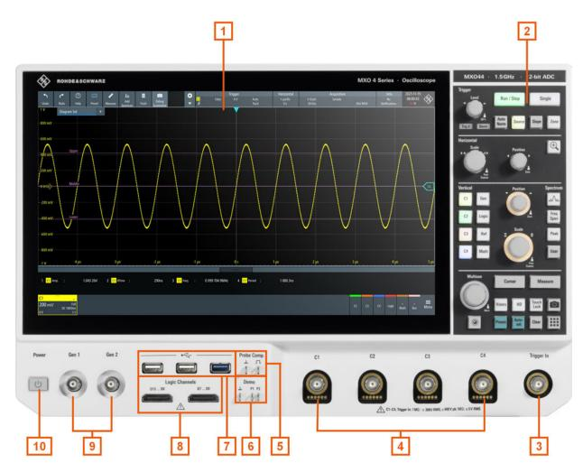
Figure 3-1: Front panel of R&S MXO 4
