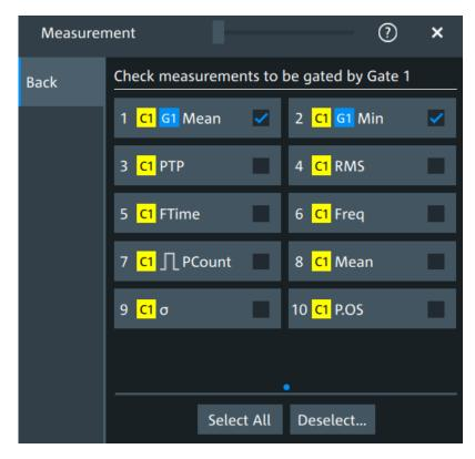
Figure 9-1: Automatic measurements gate dialog
