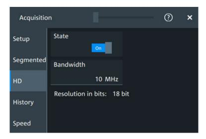
High definition is a special acquisition mode of the oscilloscope. This mode has only one setting - the filter bandwidth.
