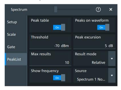
In the peak list dialog, you can define various criteria for a peak search. The peaks can be indicated in the frequency diagram by peak boxes, and the measured peak frequencies and magnitudes are listed in the peak list table.
