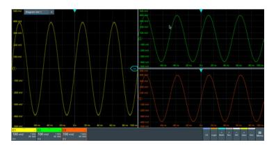
//Add zoom to C3. The zoom is located in diagram 3.  $\label{eq:located} \mbox{LAY:ZOOM:ENAB 1}$   $\mbox{LAY:ZOOM:SOUR 3}$
