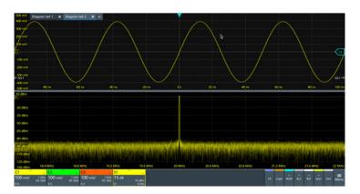
//Set C1 and spectrum side by side by changing the split type.  ${\tt LAY2:NODE1:STYP\ HOR}$
