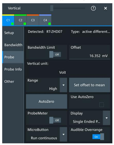
Figure 6-6: Setup for high-voltage differential probe R&S RT-ZHD07
