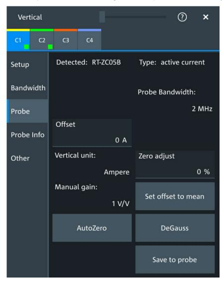
Figure 6-7: Setup for current probe R&S RT-ZC05B
