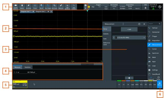
Figure 4-6: Control elements on the graphical user interface
