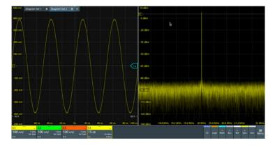
//Add zoom to spectrum. The zoom is located in layout 2, in diagram 2.  $\label{lay2:ZOOM:ENAB 1} {\tt LAY2:ZOOM:SOUR 2}$
