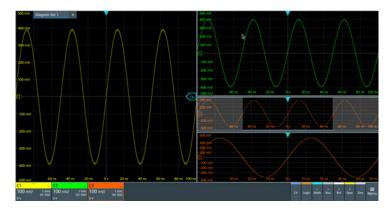
//Add a second layout with C1 and spectrum of C1. //By default, the new layout is empty. LAY2:ENAB 1
