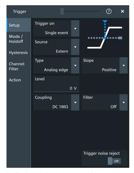
The "Slope" and "Level" are the same settings as for the edge trigger, see:
