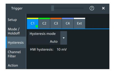
The rejection of noise by setting a hysteresis avoids unwanted trigger events caused by noise oscillation around the trigger level.
