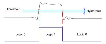
By default, same threshold and hysteresis value are used for all digital channels and all logic buses: "Couple thresholds" is enabled.
