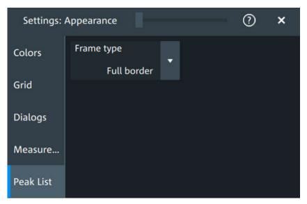
Peak list settings apply to peak list measurements. They are visible when the peak list for spectrum measurements is enabled.
