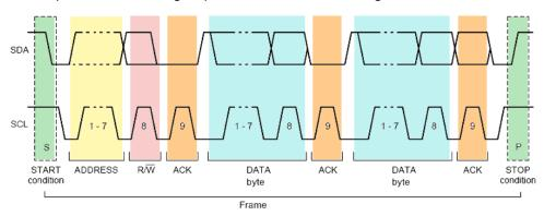
Figure 13-5: I2C writes access with 7-bit address
