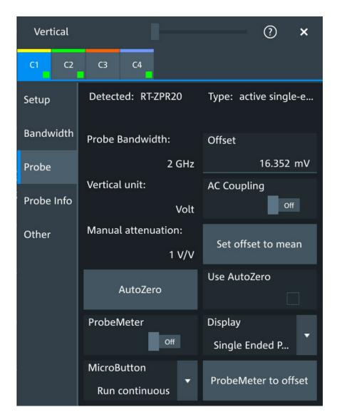
Figure 6-5: Probe setup for power rail probe R&S RT-ZPR20
