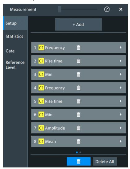
3. Tap on the button of the measurement that you want to delete. Alternatively, tap "Delete All" to delete all measurements.
