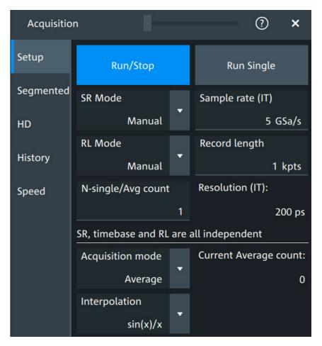
Figure 6-2: Acquisition settings: manual sample rate and record length
