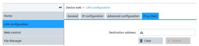
To initiate a ping between the compliant instrument and a second connected device:
