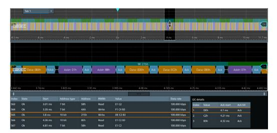
Figure 13-8: Decoded I2C signal, and decode results
