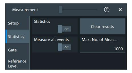
In addition to the current measurement results, you can enable a statistical evaluation. It returns the current, minimum and maximum measurement values, the average and standard deviation, and the number of measured waveforms. The results are shown in a separate tab below the grid. If the cursor measurement is active simultaneously, its results are shown beside the statistics results.
