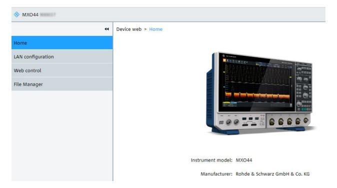
The instrument homepage displays the device information in read-only format, including DNS host names and the VISA resource string.
