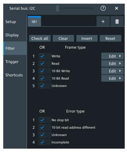
In the "Filter" tab, you can define the settings to display only the frames that match the selected filter conditions.
