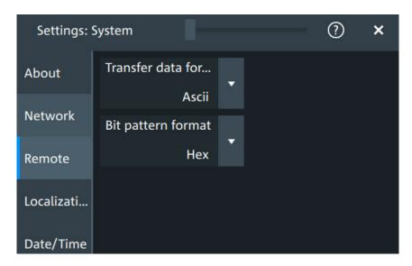
The following settings are required for remote control of the instrument via a connected computer.
