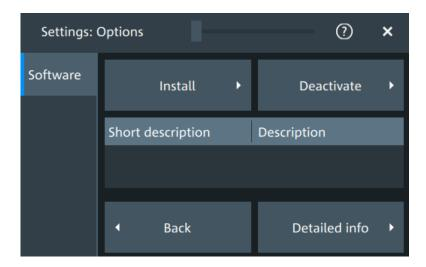
In this dialog, you can access settings for installing and deactivating options. In the "Detailed Info" dialog, you can get an overview of all options installed on your R&S MXO 4.
