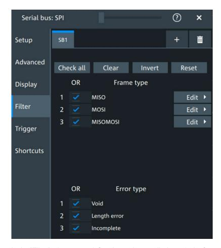
In the "Filter" tab, you can define the settings to display only the frames that match the selected filter conditions.
