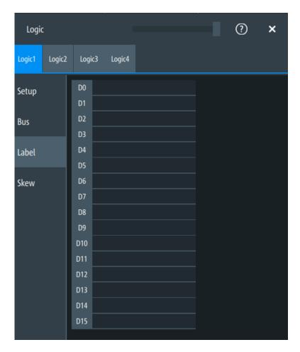
In this tab, you can enter a name for each digital channel. The name is displayed in the diagram.
