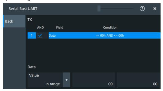
"Field" Enables the field type that you want to filter on for the selected frame.
