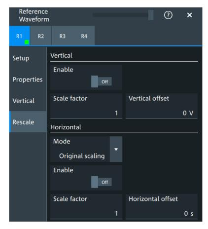
In the "Rescale" tab you can adjust the vertical and horizontal scaling of the reference waveform.
