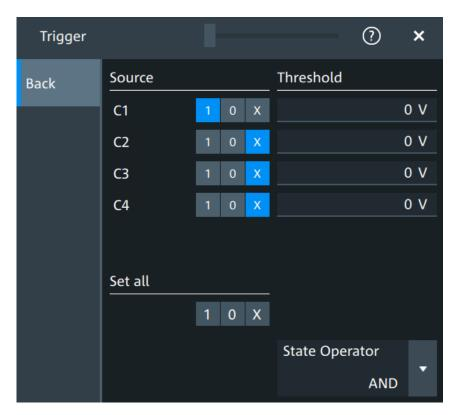
Figure 7-3: Set state for pattern trigger
