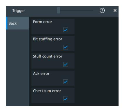
"Form error" A form error occurs when a fixed-form bit field contains one or more illegal bits.
