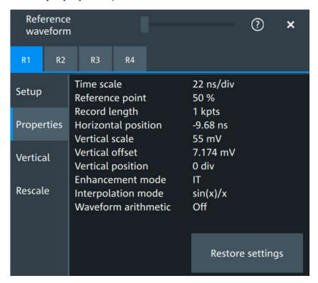
A reference waveform can be scaled, stretched and positioned in the diagram. The "Properties" tab shows the original settings of the reference waveform, which are stored together with the waveform data.
