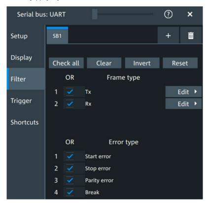
In the "Filter" tab, you can define the settings to display only the frames that match the selected filter conditions.
