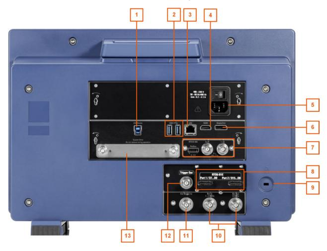
Figure 5-2: Rear panel of R&S RTO6
