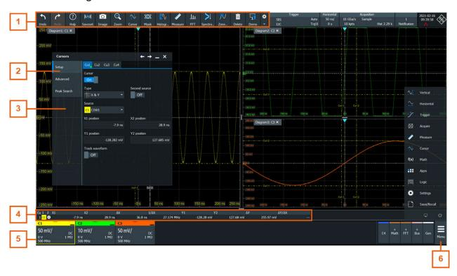
Figure 6-6: Control elements on the touchscreen
