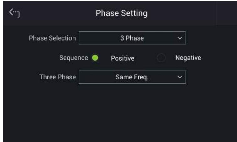
When a 3-phase balance is in use, you may set the output voltage to be Phase Volt or Line Volt. Below is the procedure for setting the 3-phase voltage output to a 3-phase balance.
