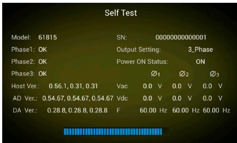
During initialization, the Regenerative Grid Simulator executes memory, data, and communication self-tests. The display shows the Model Number and Regenerative Grid Simulator's Serial Number after executing the self-test routines and each test item will show "OK" on the right if no error is found. The software version will show on the display.
