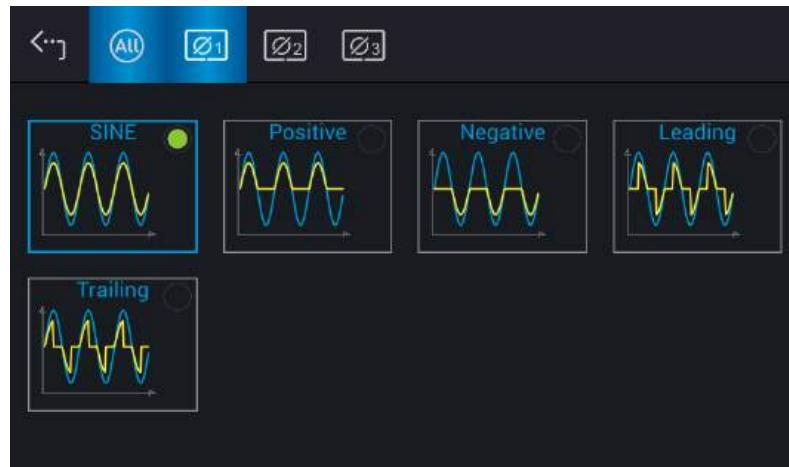
Set the 3-phase waveform to the leading edge wave at the same time:
