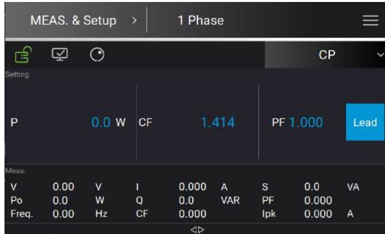
When set to Lead, it means that the current loading phase leads to the UUT voltage phase. When set to Lag, it means the current loading phase lags behind the UUT voltage phase.
