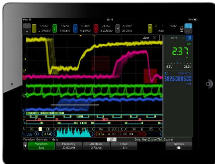
Figure 53. Controlling the 6000 X-Series via tablet device.
