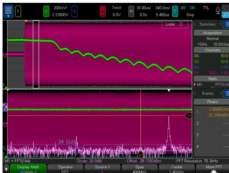
Figure 37a. Gated FFT time correlating the PLL voltage, SPI command and spectrum content at a given time span.
