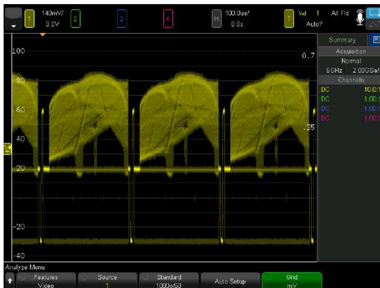
Figure 45. Triggering on a 1080p/60 signal.
