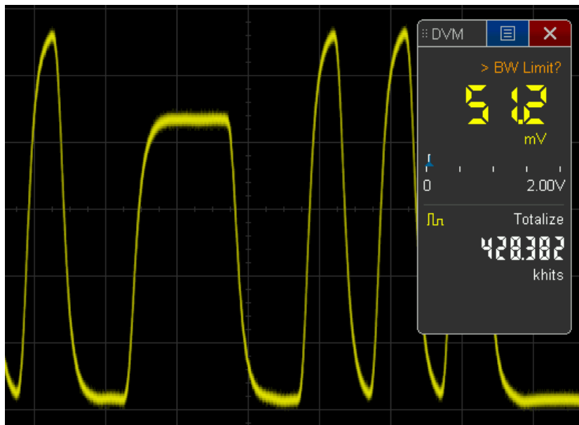
Figure 35. Totalizing the number of runt errors.
