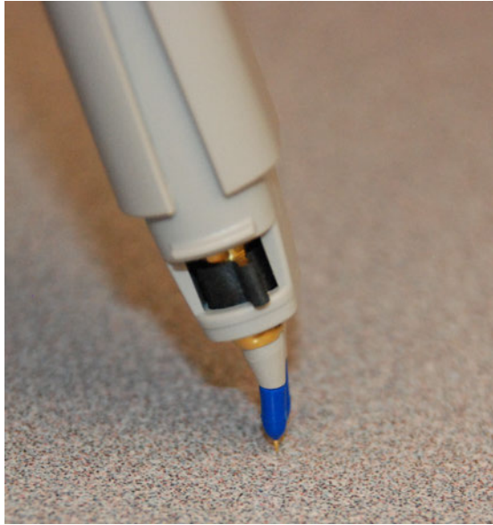
Figure 28 Proper Vertical Orientation of the Blue Tips
