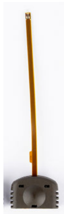
Discoloration after usage under high temperatures
