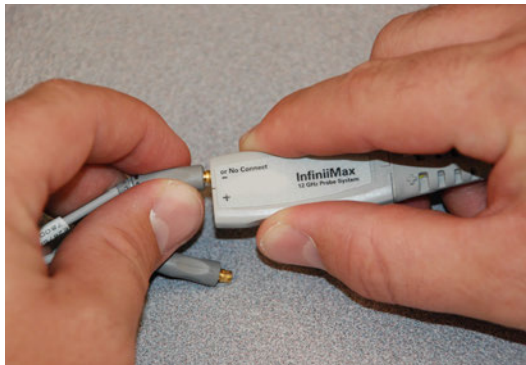
Figure 4 Properly Pulling the Probe Head Straight Out
