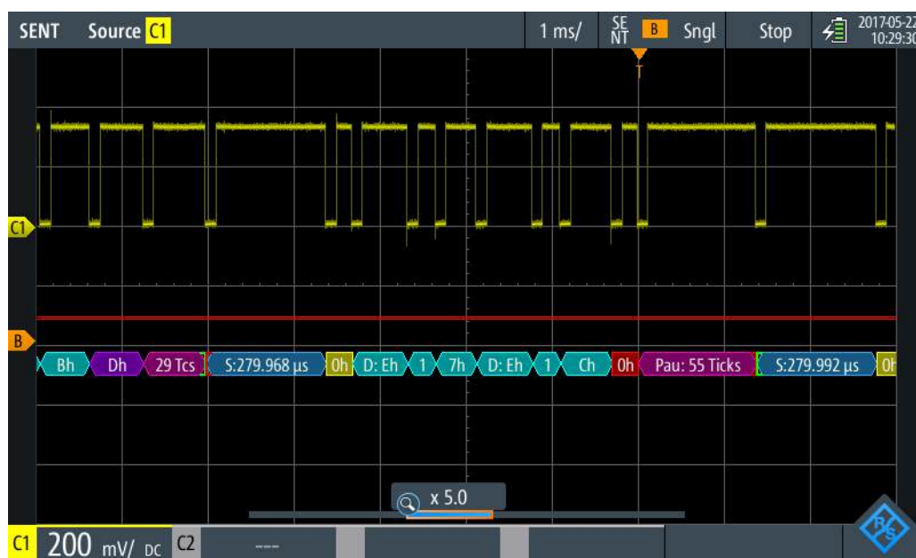
Figure 9-44: Comb display of a decoded SENT signal, triggered on fast CRC
