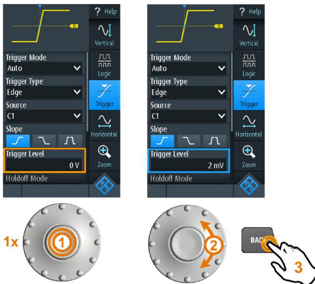
Figure 2-10: Set numerical values using the wheel
