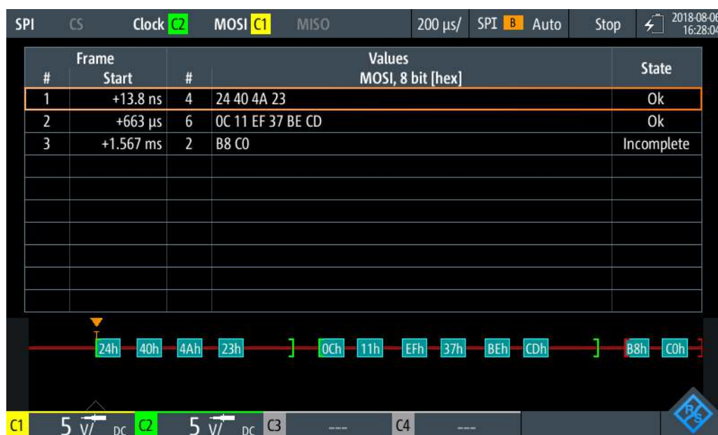
Figure 9-18: Decoded SPI signal in Protocol mode
