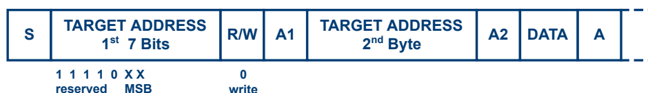
Figure 9-8: 10-bit address, write access
