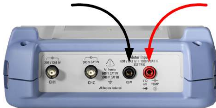
Figure 7-1: Meter inputs to connect test leads
