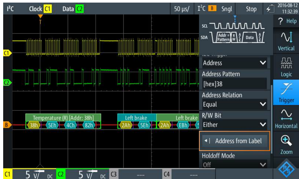
Figure 9-11: Trigger on address "Temperature", value 38 (hex)
