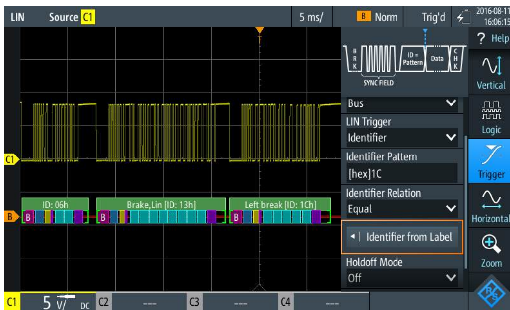
Figure 9-36: Trigger on identifier "Left brake"
