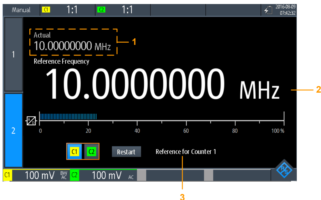
Figure 11-2: Display for reference counter
