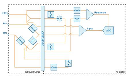
The NI 9984 and NI 9985 provide a quarter-bridge completion resistor and half-bridge completion resistors.
