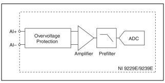
Figure 5. Input Circuitry for One Channel of the NI 9229E/9239E
