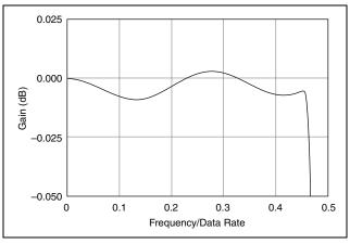
Figure 6. Typical Passband Flatness for the NI 9229E/9239E
