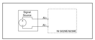
Figure 4. Connecting a Floating Signal Source to the NI 9229E/9239E
