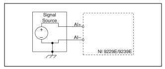
Figure 3. Connecting a Grounded Signal Source to the NI 9229E/9239E
