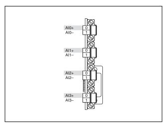
Figure 2. NI 9229E/9239E Terminal Assignments
