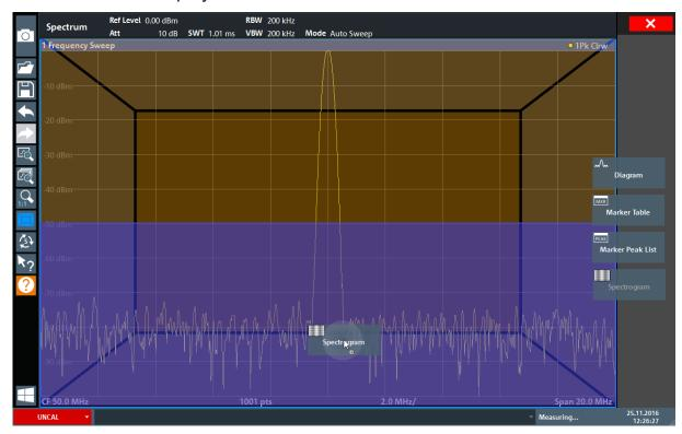
Figure 6-3: Adding a Spectrogram to the display
