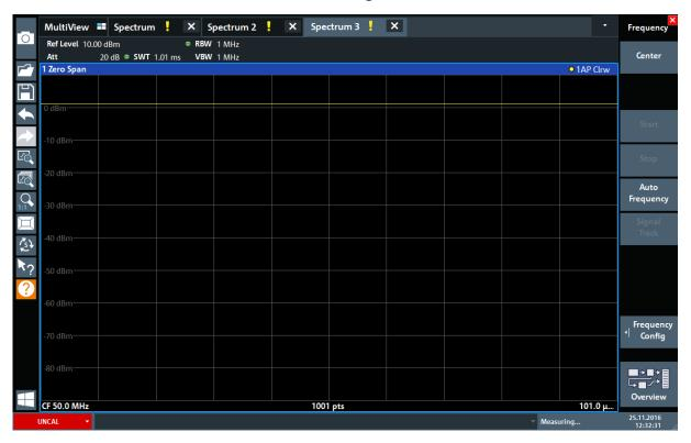
Figure 6-7: Time domain display of the calibration signal
