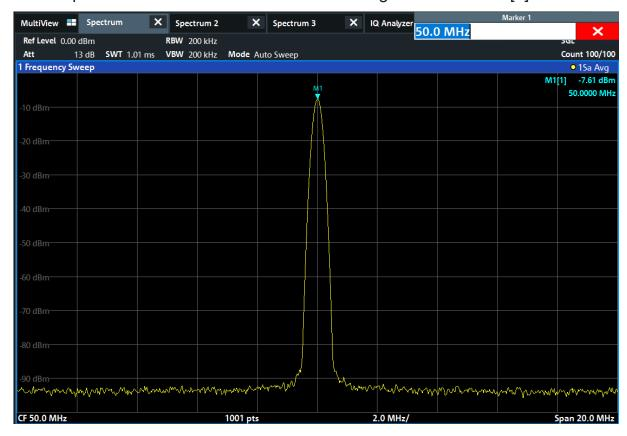
6. Now you can move the marker by tapping and dragging it to a different position. The current position is indicated by a dotted blue line. Notice how the position and value change in the marker area of the diagram.
