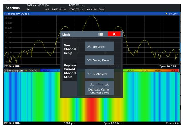
Figure 6-5: Adding a new measurement channel
