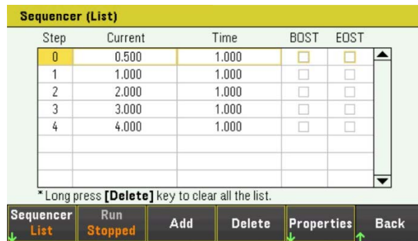
Figure 12. A List generates a complex sequence of changes with rapid and precise timing input
