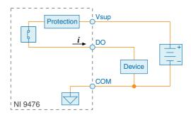
The NI 9476 has sourcing outputs. Sourcing outputs drive current from Vsup to DO when the channel is on.
