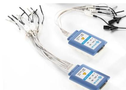
The digital inputs are grouped into logic probes with eight channels. High input impedance combined with low input capacitance of 100 kΩ II 4 pF ensures high signal fidelity and low loading of the test points.
