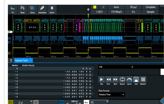
Use the digital channels to decode parallel buses. These are displayed in a digital bus format or as an analog waveform. For clocked parallel buses, the decoded contents can also be displayed in a table. In addition, you can use the digital channels of the R&S RTx-B1 option to decode serial interface protocols such as SPI and I<sup>2</sup>C.
