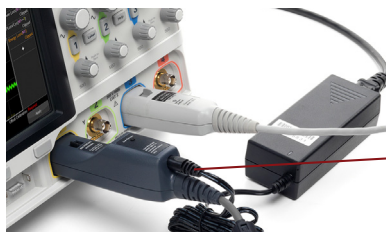
External power supply plugged into N7026A
