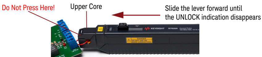
Figure 6 Use the Opening Lever
