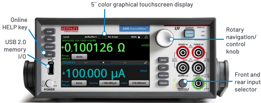
2450 front panel with high-resolution, capacitive touchscreen.
