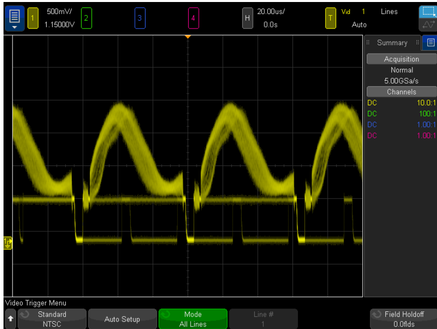
Figure 30 Triggering on All Lines
