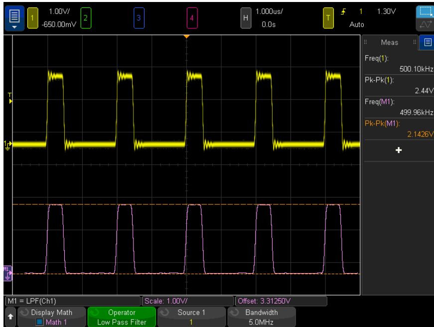
Figure 16 Example of Low Pass Filter
