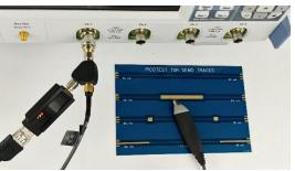
The Picotest TDR Demo Trace test board provides four sample traces; 50 ohm, Beatty trace, 50 Ohm with 3" markers notches, and 50 to 52.5 ohm to 50 Ohm. The resistive splitter is included and supports TDR/TDT operation.
