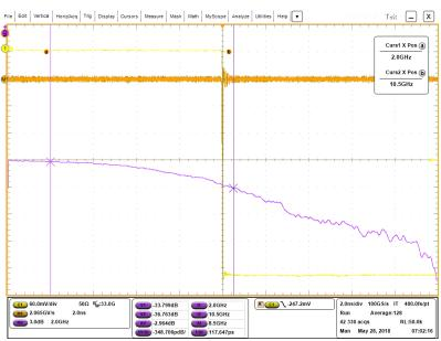
The -3dB bandwidth of the PerfectPulse edge is 10.5 GHz while it is - 0.6dB at 5GHz and -0.1dB at 2GHz
