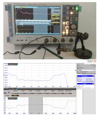
Using the TDR function, along with the Picotest P2100A 50 ohm PDN probe for injection, you can test PCB coupon impedance. This image shows the change from 47 to 51 Ohms.
