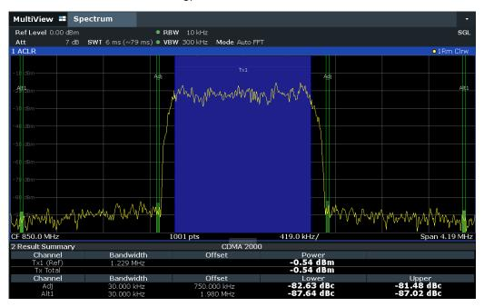
Results are provided for the TX channel and the number of defined adjacent channels *above and below* the TX channel. If more than one TX channel is defined, you must specify the channel to which the relative adjacent-channel power values refer. By default, it is the TX channel with the maximum power.
