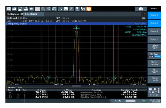
All markers can be defined as band power markers, each with a different span. When a band power marker is activated, if no marker is active yet, marker 1 is activated. Otherwise, the currently active marker is used as a band power marker (all other marker functions for this marker are deactivated).
