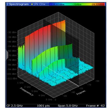
Figure 6-61: Three-dimensional spectrogram
