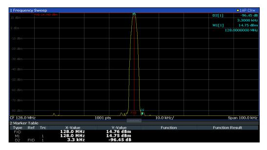
You can move the position of the fixed reference marker graphically by dragging the display lines, or numerically by entering values for the marker position and level.
