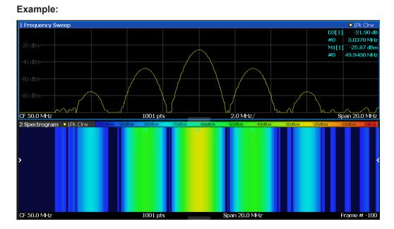
In this example, you see the spectrogram for the calibration signal of the R&S FPL1000, compared to the standard spectrum display. Since the signal does not change over time, the color of the frequency levels does not change over time, i.e. vertically. The legend above the spectrogram display describes the power levels the colors represent.
