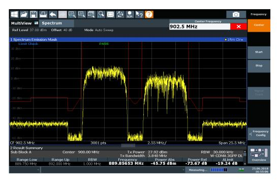
Figure 6-30: Summarized limit line for multiple sub blocks
