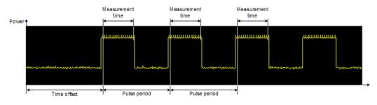
To get a valid result, you have to perform a complete measurement with synchronization to the end of the measurement before reading out the result. This is only possible for single sweep mode.
