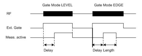
Figure 6-51: Effects of Gate mode, Gate delay and Gate length
