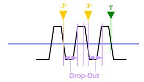
Figure 6-49: Trigger drop-out time for falling edge trigger
