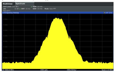
Figure 6-52: GSM signal with GATE OFF
