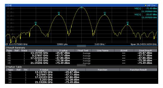
Figure 6-40: EMI measurement results
