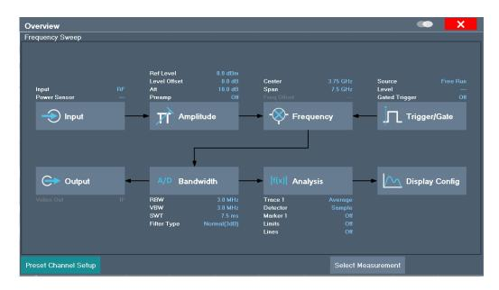
Using this overview, you can easily configure an entire channel setup from input over processing to output and analysis by stepping through the dialog boxes as indicated.
