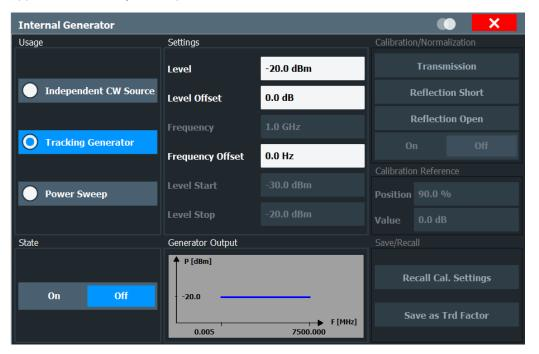
The preview in the dialog box visualizes the configured signal from the internal tracking generator.
