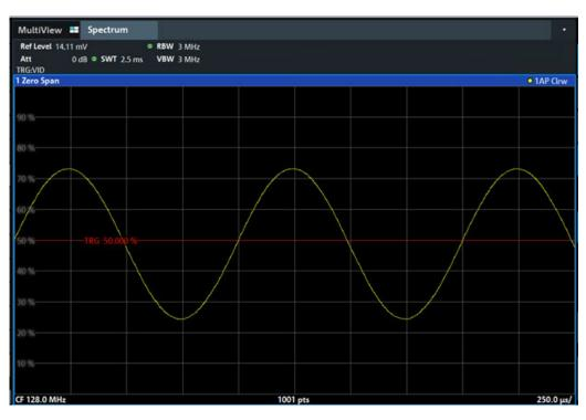
Figure 6-10: Measurement of the AM modulation depth
