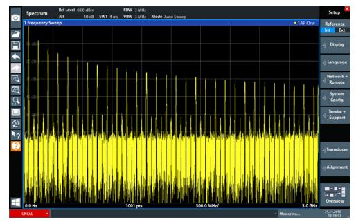
Figure 4-4: Calibration signal as RF input
