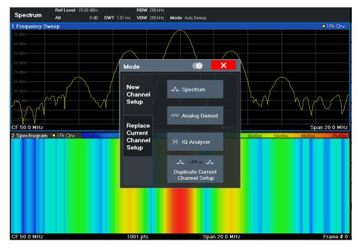
Figure 4-8: Adding a new measurement channel
