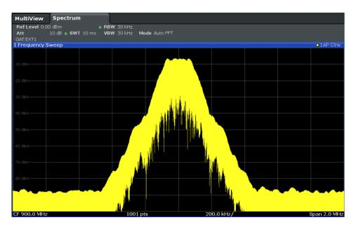
Figure 6-53: GSM signal with GATE ON
