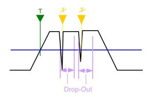
Figure 6-48: Effect of the trigger drop-out time
