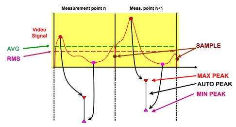
You can define the trace detector to be used for the individual traces manually, or the R&S FPL1000 can select the appropriate detector automatically.
