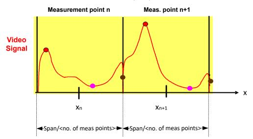
Using the bin-centered method, the first and last x-values of the trace are not identical to the exact starting and end point of the measurement span. The distance between two sweep points corresponds to the width of the bin, or span/(<no\_sweep\_points>).
