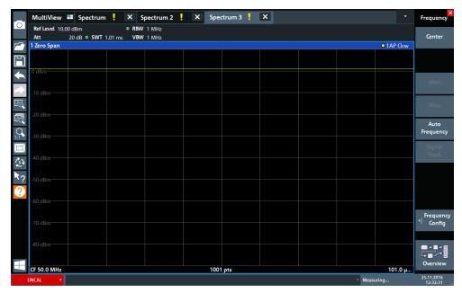
Figure 4-10: Time domain display of the calibration signal
