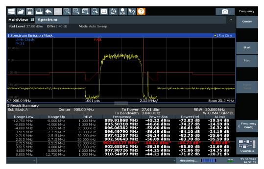
The indicated limit line depends on the settings in the "Sweep List". Several types of limit checks are possible:
