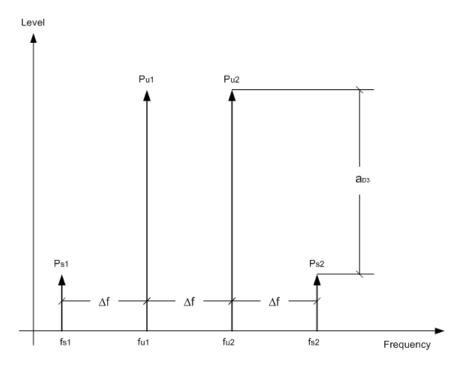
Figure 6-36: Intermodulation products Ps1 and Ps2
