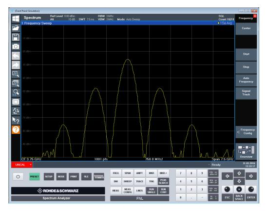
To hide or show the front panel temporarily, press the [F6] key on the external keyboard (if available) or the remote computer.
