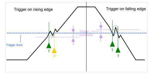
Figure 6-47: Effects of the trigger hysteresis
