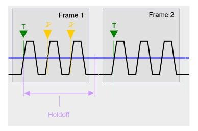
Figure 6-50: Effect of the trigger holdoff
