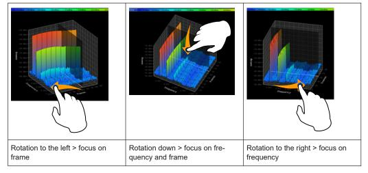
Table 6-28: Effect of rotating the spectrogram in three dimensions
