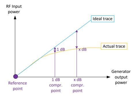
Figure 6-21: Compression point calculation
