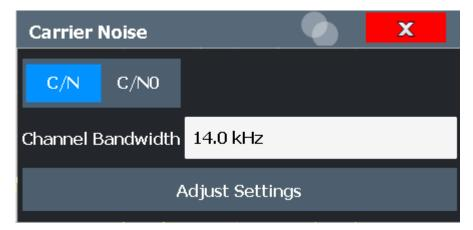
Carrier-to-noise measurements are not available in zero span mode.
