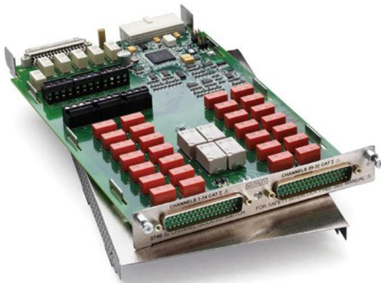
The 3740 offers 28 general-purpose form C channels that are ideal for routing power or other control devices. For higher power applications of up to 7 A, four additional high current form A channels are provided.
