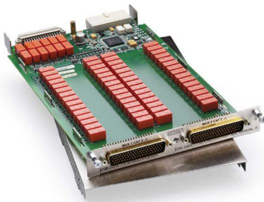
The 3720 offers two independent banks of 1x30 two-pole multiplexers. It is ideal for general purpose switching, including temperature measurements. The two banks can automatically be connected to the Series 3700A mainframe backplane and optional DMM through the analog backplane connection relays. This connection allows the mainframe to reconfigure the card to a single 1x60 two-pole multiplexer or to enable card-to-card expansion for even larger configurations.
