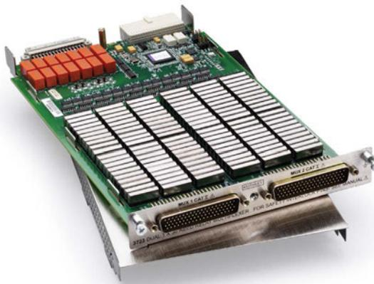
The 3723 offers two independent banks of high speed 1x30 two-pole multiplexers that are ideal for high speed scanning applications. The two banks can automatically be connected to the Series 3700A mainframe backplane and optional DMM through the analog backplane connection relays. This connection allows the mainframe to reconfigure the 3723 as a single 1x60 two-pole multiplexer or as a single 1x120 single-pole mode. It also enables card-to-card expansion for even larger configurations.
