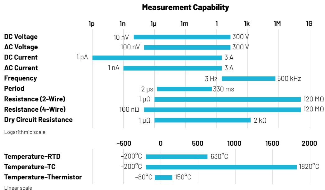
Measurement capabilities of the high performance multimeter
