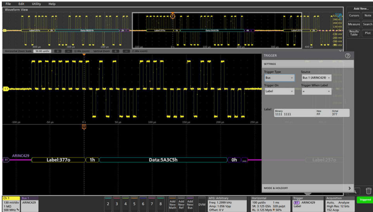
Decoded ARINC 429 bus, with the acquisition triggered on a specified label value.
