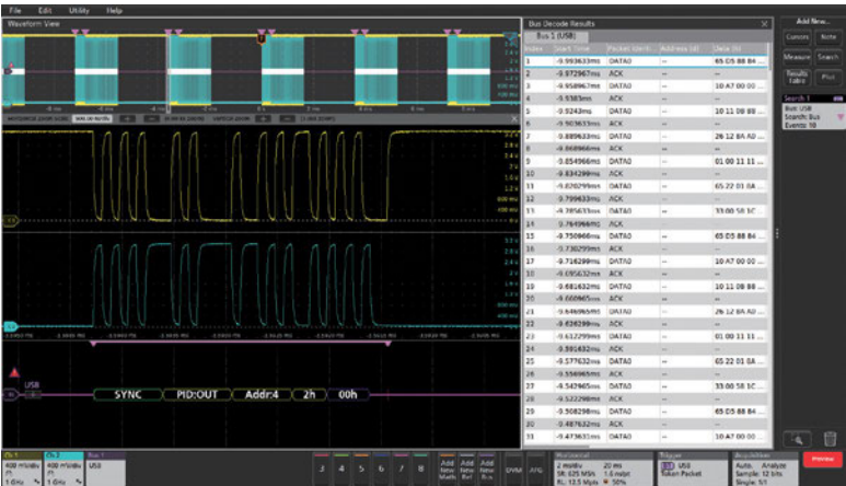
Serial protocol trigger / analysis (optional). Support is available for most common serial bus standards.
