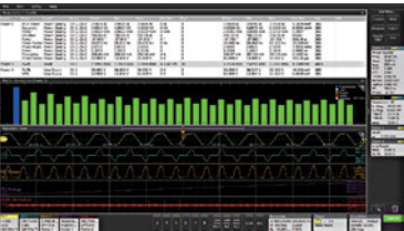
Power analysis packages enable automatic measurement of harmonics, switching loss and other key parameters.
