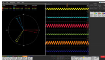
Debug motor drive designs by viewing the drive input/output voltage and current signals with waveforms and phasor diagrams.
