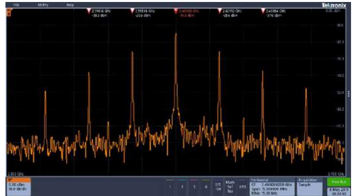
Figure 9: Automated peak markers identify critical information at a glance. As shown here, the five highest amplitude peaks that meet the threshold and excursion criteria are automatically marked along with each peak's frequency and amplitude.
