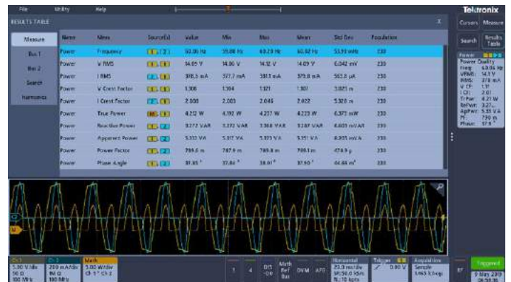
Figure 7: Power Quality measurement table. Automated power measurements enable quick and accurate analysis of common power parameters.
