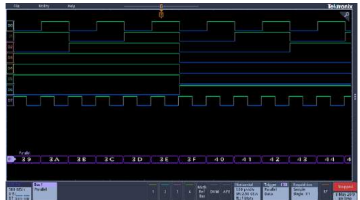
Figure 17: With color-coded digital waveform display, groups are created by simply placing digital channels together on the screen, allowing digital channels to be moved as a group.
