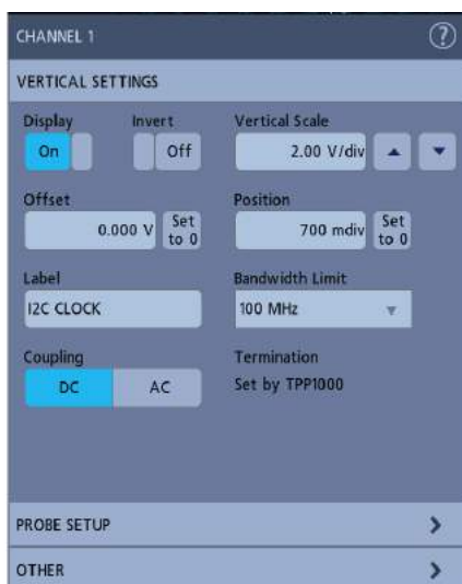
Figure 1: Configuration menus are accessed by simply double-tapping on the item of interest on the display. In this case, the Channel badge was double-tapped to open the channel configuration menu. Menus are dismissed by simply tapping outside of them.
