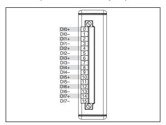
Figure 2. NI 9422 Terminal Assignments
