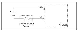
Figure 3. Connecting a Sinking-Output Device to the NI 9422
