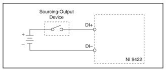
Figure 4. Connecting a Sourcing-Output Device to the NI 9422
