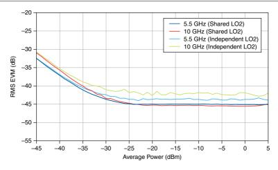
Figure 18. IF 5G NR 2 CC x 400 MHz RMS EVM versus Average Power, Measured 14, 18
