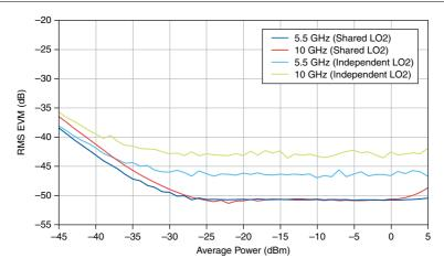
Figure 16. IF 5G NR 2 CC x 100 MHz RMS EVM versus Average Power, Measured 14,16
