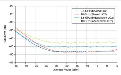
Figure 17. IF 5G NR 1 CC x 400 MHz RMS EVM versus Average Power, Measured 14, 17
