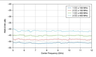
**Figure 20.** IF 5G NR RMS EVM versus Frequency (Independent LO2), Measured<sup>14, 19, 20</sup>
