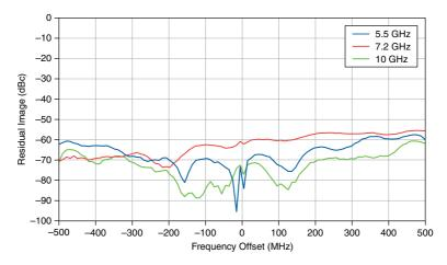
Figure 7. Maximum IF Output Residual Sideband Image Versus Upconverter Center Frequency, Measured
