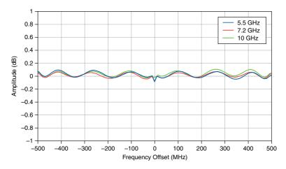
Figure 9. Maximum IF Input Frequency Response Deviation versus Downconverter Center Frequency, Measured
