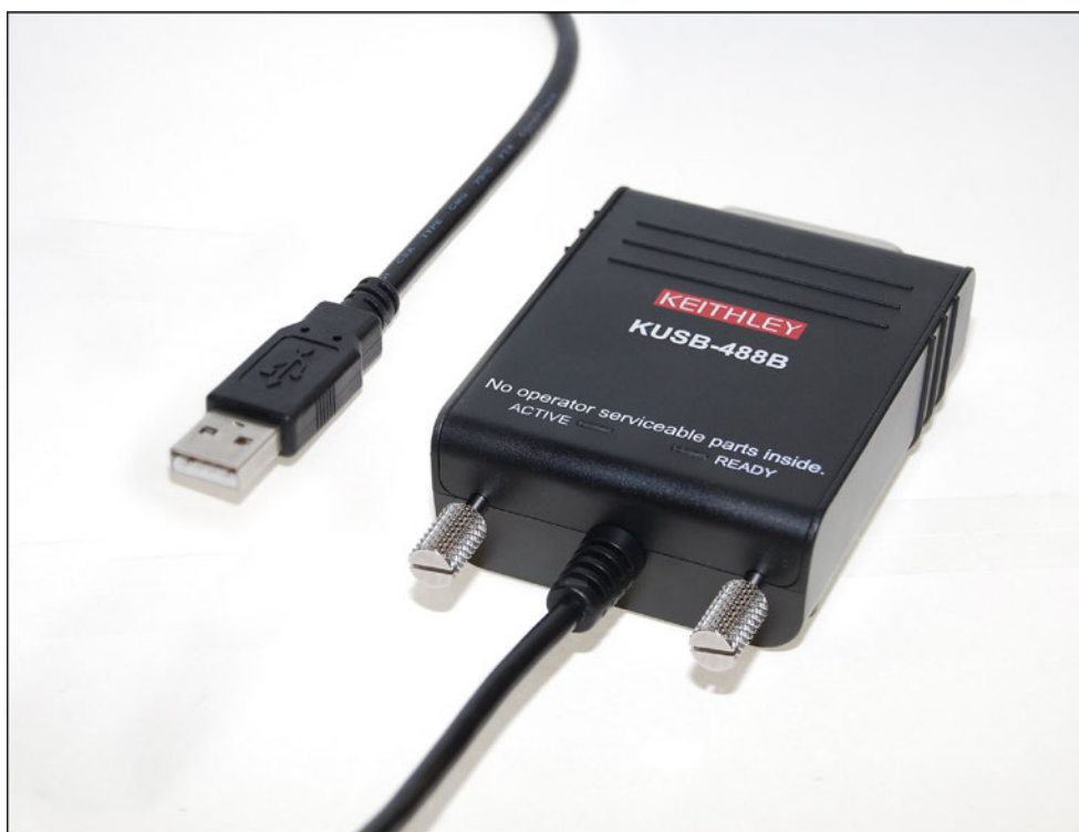
Figure 1: KUSB-488 USB to GPIB converter
