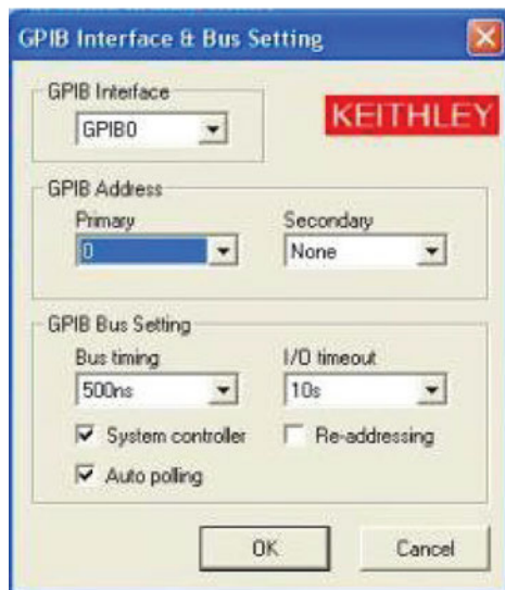
Figure 5: GPIB interface and bus configuration
