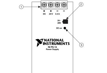
Figure 1-2. Front View of the NI PS-14 Power Supply
