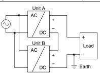
Figure 2-2. NI PS-14 in Serial Operation
