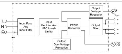
Figure 1-1. Functional Diagram for the NI PS-14 Power Supply
