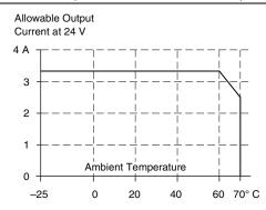
Figure A-14. Output Current Vs. Ambient Temperature
