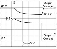
Figure 2-4. Peak Current Capacity Output Voltage Dips
