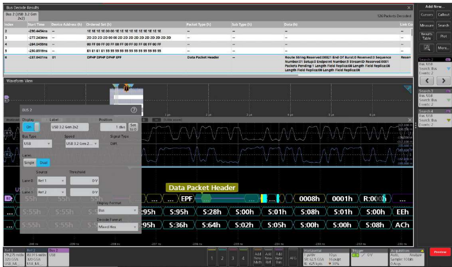
Bus configuration for the USB bus with decode speed USB 3.2 Gen2x2 for the DP packets. Search on packet type LMP along with lane 0 and lane 1 search on training sequence is added.
