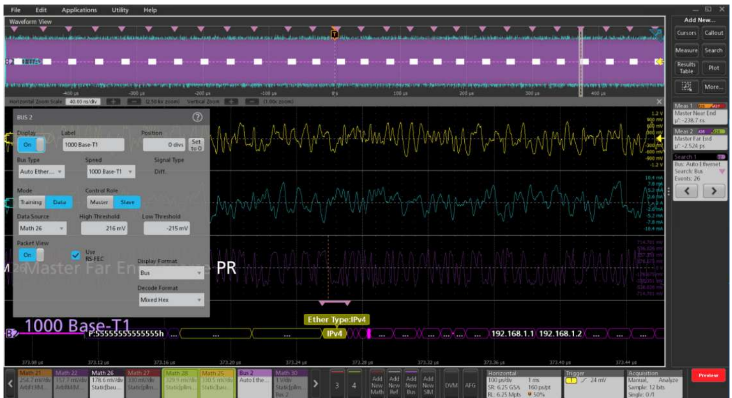
1000baseT1 full duplex signals on Ch1 and Ch2. Math 26 shows the separated signal.
