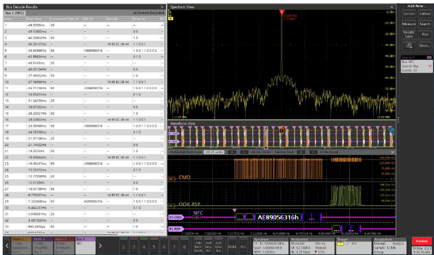
The results table provides time-stamped, tabular view of all captured packets on the NFC bus. 33 occurrences of the event is searched on SOC on the command lane.
