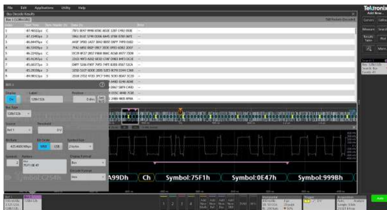
128B132B bus showing decode with MSB. Symbol was searched with 41 occurrences.
