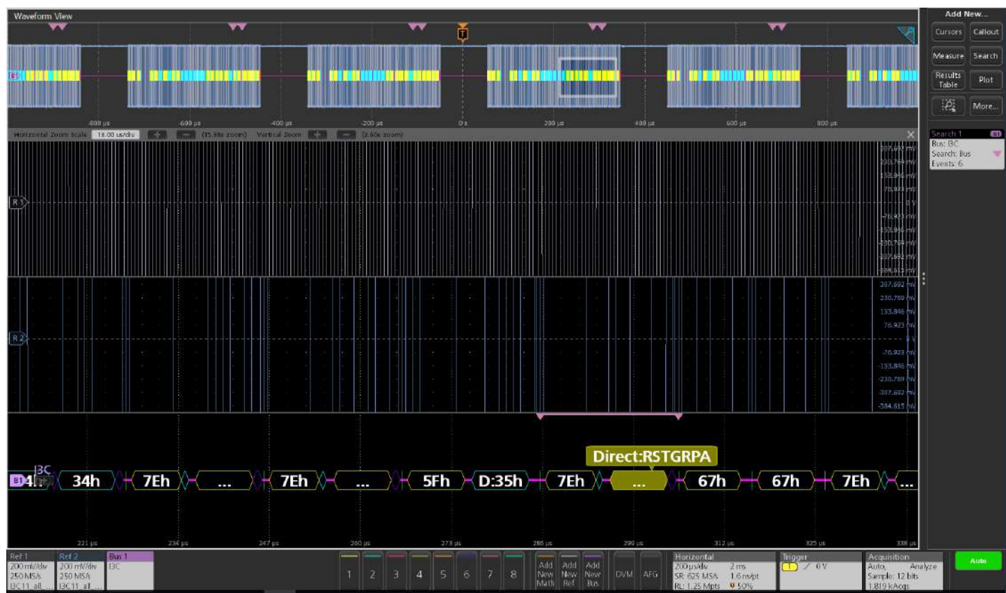
Searching the I3C bus with decode version 1.1 for the packet with Reset Group Address.
