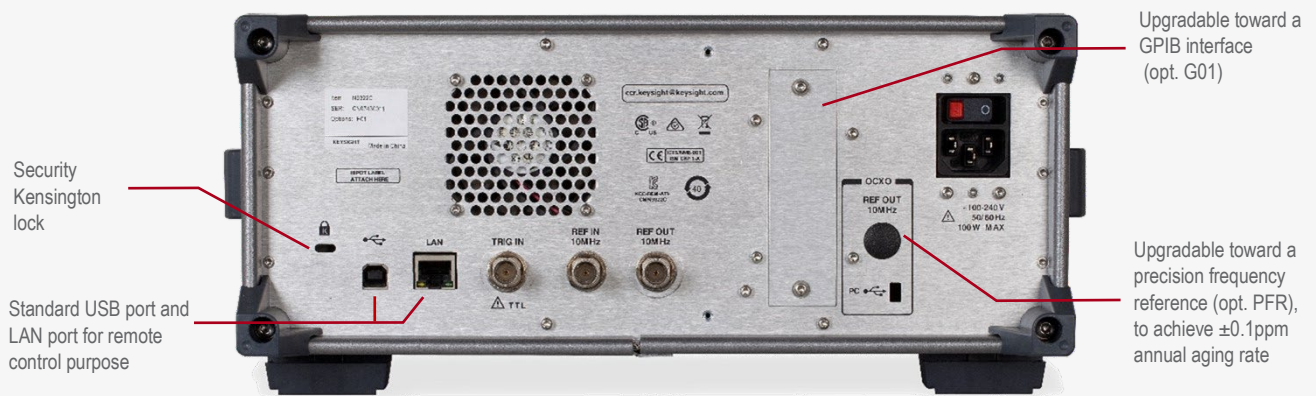
Figure 5. The rear panel of N932xC spectrum analyzer
